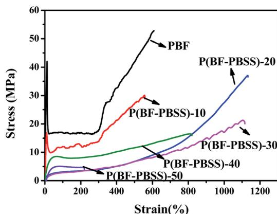
Fig. 7 Strain–stress curves of PBF and P(BF-PBSS)s.
