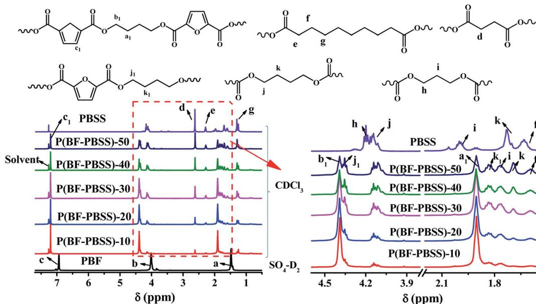
Fig. 1  $^1\text{H}$ -NMR spectra of PBF and P(BF-PBSS)s.
