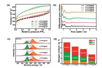
Fig. 2 (a) Nitrogen adsorption/desorption isotherm and (b) pore size distributions for p-PYPZs; (c) Overall XPS analysis scanned spectrum of p-PYPZs; (d) high resolution N 1s XPS spectra of p-PYPZs.
