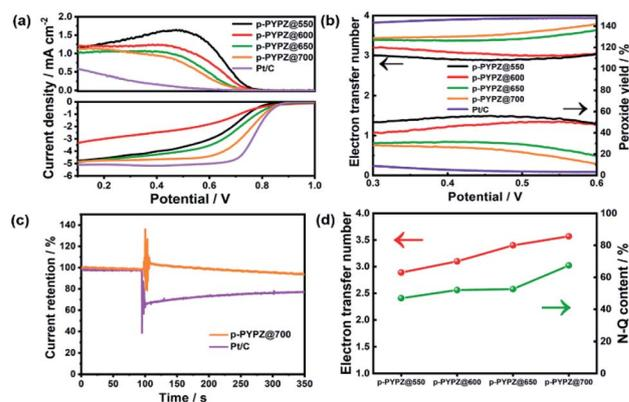
Fig. 5 (a) RRDE voltammogram curves of *p*-PYPZs samples and Pt/C recorded in 0.1 M KOH at 1600 rpm and 5 mV s<sup>-1</sup>; (b) electron transfer number and peroxide yield rate calculated from the RRDE tests; (c) methanol-tolerance test for *p*-PYPZ@700 and commercial Pt/C; (d) electron transfer number *n* and N-Q content.
