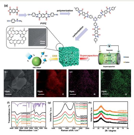
Fig. 1 (a) Schematic of the synthesis of p-PYPZg(b) SEM image of p-PYPZg600; (c-e) SEM-EDS mapping images of p-PYPZg600; (f) FT-IR spectra of PYPZ and p-PYPZs; (g) Raman spectra of p-PYPZs; and (h) XRD patterns of p-PYPZs.
