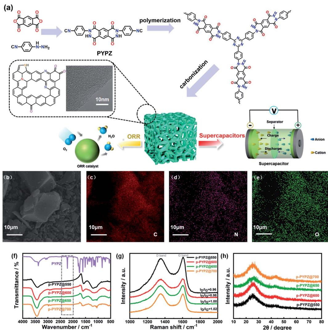
Fig. 1 (a) Schematic of the synthesis of *p*-PYPZs; (b) SEM image of *p*-PYPZ@600; (c–e) SEM-EDS mapping images of *p*-PYPZ@600; (f) FT-IR spectra of PYPZ and *p*-PYPZs; (g) Raman spectra of *p*-PYPZs; and (h) XRD patterns of *p*-PYPZs.
