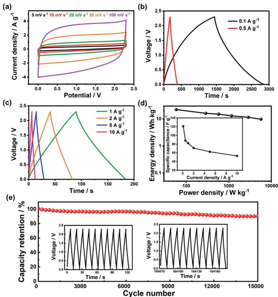
Fig. 4 Electrochemical performance of *p*-PYPZ@600 in the two-electrode system with TEABF<sub>4</sub>/AN: (a) CV curves at different scan rates; (b) GCD curves at 0.1 A g<sup>-1</sup> and 0.5 A g<sup>-1</sup>; (c) GCD curves at 1, 2, 5, and 10 A g<sup>-1</sup>; (d) Ragone plots (inset: specific capacitance at different current densities); (e) long-term cycling tests of the *p*-PYPZ@600 electrode with the electrolyte of TEABF<sub>4</sub>/AN (inset: GCD curves for the first and last 10 cycles).
