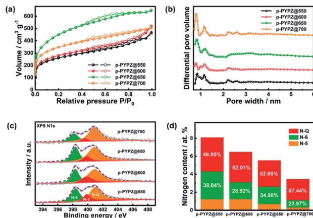
Fig. 2 (a) Nitrogen adsorption/desorption isotherm and (b) pore size distributions for *p*-PYPZs; (c) Overall XPS analysis scanned spectrum of *p*-PYPZs; (d) high resolution N 1s XPS spectra of *p*-PYPZs.
