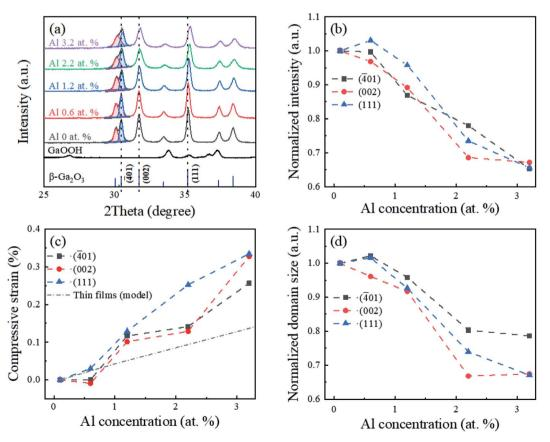
Fig. 1 (a) XRD patterns of GaOOH and  $\beta$ -Ga<sub>2</sub>O<sub>3</sub> nanostructures with different Al concentrations; the bottom ticks indicate PDF Card No. 01-076-0573 for  $\beta$ -Ga<sub>2</sub>O<sub>3</sub>. (b) Normalized peak intensity, (c) compressive strain, and (d) normalized domain size of (-401), (002), and (111) planes as a function of Al concentrations. The compressive strain in this work was compared with that of the thin film (model).<sup>29</sup>
