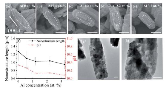
Fig. 2 (a-e) SEM images (scale bar: 500 nm) and (f) average length of β-Ga<sub>2</sub>O<sub>3</sub> nanostructures with increasing Al concentrations. TEM images (scale bar: 100 nm) of (g) GaOOH nanostructures (before annealing) and (h) β-Ga<sub>2</sub>O<sub>3</sub> nanostructures (after annealing) without Al doping.
