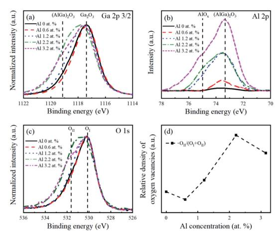
Fig. 4 XPS analysis of  $\beta$ -Ga<sub>2</sub>O<sub>3</sub> nanostructures with different Al concentrations: core-level spectra of (a) Ga  $2p_{3/2}$ , (b) Al 2p, and (c) O 1s. The XPS intensity in (a and c) is normalized to increase clarity. (d) Relative intensity of  $O_{II}/(O_I + O_{II})$  in O 1s spectra as a function of Al concentrations. The peak energies were calibrated using an adventitious C 1s of 284.68 eV.
