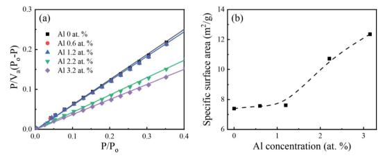
Fig. 3 (a) BET surface area plot for Al-doped  $Ga_2O_3$  nanostructures with different Al concentrations and (b) specific surface area as a function of Al concentrations; Va, Po, P, and P/Po are the adsorbed gas quantity, saturation pressure of the adsorbate, equilibrium pressure of the adsorbate, and relative pressure, respectively.
