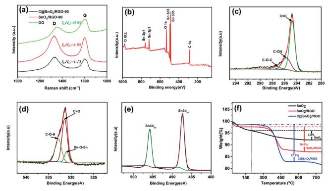
Fig. 3 (a) Raman spectrum of the  $C@SnO_2/RGO-90$ ,  $SnO_2/RGO-90$ , GO composite and (b) full survey XPS spectrum of the  $C@SnO_2/RGO-90$  composite, (c-e) high-resolution XPS spectra of C1s, O1s, and Sn 3d of the  $C@SnO_2/RGO-90$ , respectively, and (f) TGA curves of  $SnO_2/RGO-90$ , and  $C@SnO_2/RGO-90$ .
