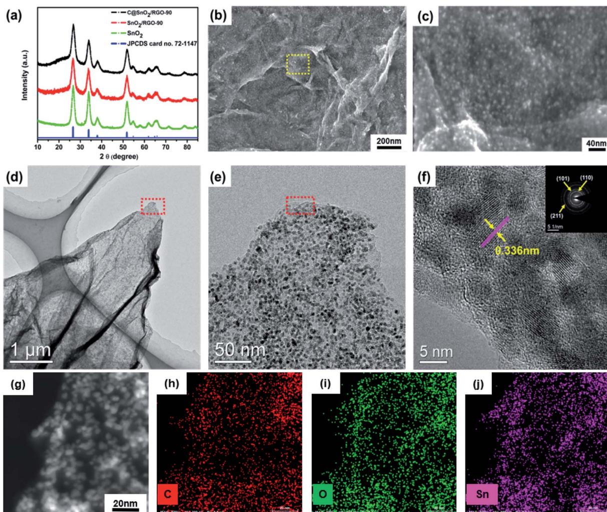
Fig. 2 (a) XRD patterns of pure SnO<sub>2</sub>, SnO<sub>2</sub>/RGO-90, and C@SnO<sub>2</sub>/RGO-90. (b and c) SEM images and (d–f) TEM images of C@SnO<sub>2</sub>/RGO-90. (g) The corresponding EDX elemental mappings (h) C, (i) O and (j) Sn of the C@SnO<sub>2</sub>/RGO-90 composite.
