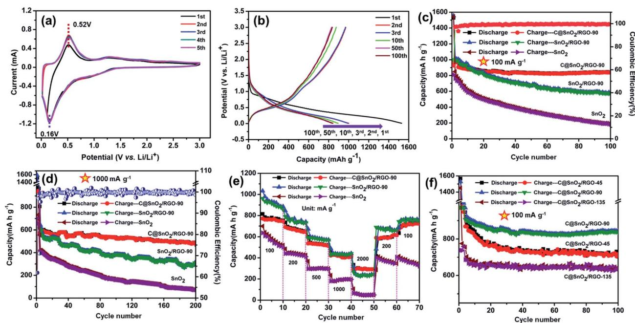
Fig. 4 (a) CV curves of C@SnO<sub>2</sub>/RGO-90 at a scan rate of 0.1 mV s<sup>-1</sup>. (b) Discharge/charge curves of C@SnO<sub>2</sub>/RGO-90 at 100 mA g<sup>-1</sup>. (c) Cycling performances and CE patterns of the C@SnO<sub>2</sub>/RGO-90 sample at 100 and (d) 1000 mA g<sup>-1</sup>. (e) Rate capacities of the three samples. (f) Cycling performances of C@SnO<sub>2</sub>/RGO samples with different RGO contents.
