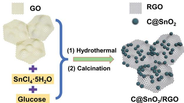
Fig. 1 Schematic illustration of the preparation of the C@SnO<sub>2</sub>/RGO composite.
