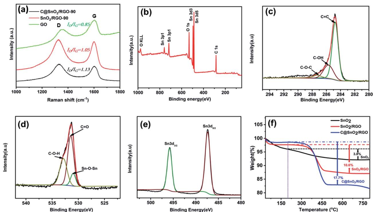
Fig. 3 (a) Raman spectrum of the C@SnO<sub>2</sub>/RGO-90, SnO<sub>2</sub>/RGO-90, GO composite and (b) full survey XPS spectrum of the C@SnO<sub>2</sub>/RGO-90 composite, (c–e) high-resolution XPS spectra of C1s, O1s, and Sn 3d of the C@SnO<sub>2</sub>/RGO-90, respectively, and (f) TGA curves of SnO<sub>2</sub>, SnO<sub>2</sub>/RGO-90, and C@SnO<sub>2</sub>/RGO-90.
