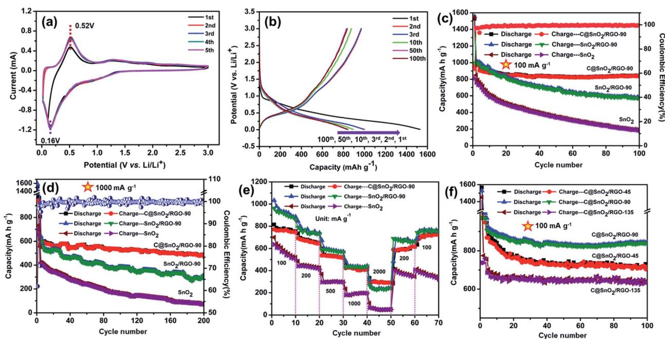
Fig. 4 (a) CV curves of C@SnO<sub>2</sub>/RGO-90 at a scan rate of 0.1 mV s<sup>-1</sup>. (b) Discharge/charge curves of C@SnO<sub>2</sub>/RGO-90 at 100 mA g<sup>-1</sup>. (c) Cycling performances and CE patterns of the C@SnO<sub>2</sub>/RGO-90 sample at 100 and (d) 1000 mA g<sup>-1</sup>. (e) Rate capacities of the three samples. (f) Cycling performances of C@SnO<sub>2</sub>/RGO samples with different RGO contents.
