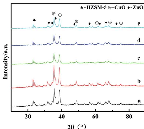
Fig. 2 XRD patterns of the catalysts: (a) CZG<sub>0</sub>H; (b) CZG<sub>1</sub>H; (c) CZG<sub>3</sub>H; (d) CZG<sub>5</sub>H; (e) CZG<sub>10</sub>H.
