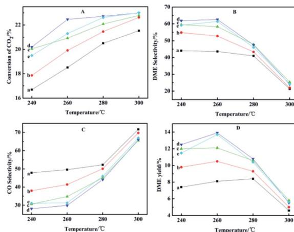
Fig. 8 Effect of reaction temperature on the catalytic performance: (a) CZG<sub>0</sub>H; (b) CZG<sub>1</sub>H; (c) CZG<sub>3</sub>H; (d) CZG<sub>5</sub>H; (e) CZG<sub>10</sub>H.
