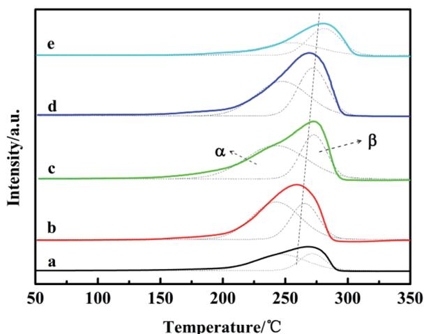
Fig. 4 H<sub>2</sub>-TPR profiles of the catalysts: (a) CZG<sub>0</sub>H; (b) CZG<sub>1</sub>H; (c) CZG<sub>3</sub>H; (d) CZG<sub>5</sub>H; (e) CZG<sub>10</sub>H.
