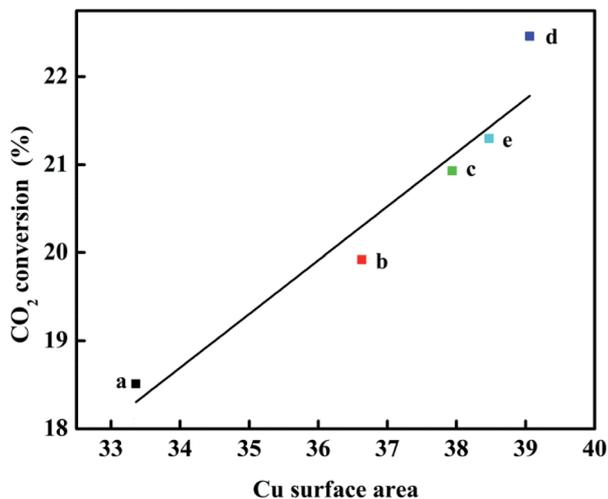
Fig. 3 Relationship between the CO<sub>2</sub> conversion and Cu surface area.
