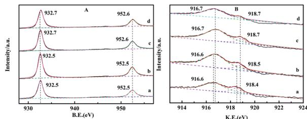
Fig. 7 Spectra of the reduced and recovered CZG<sub>0</sub>H and CZG<sub>5</sub>H hybrid catalysts: (A) Cu 2p; (B) Cu (LMM) Auger; (a) the reduced CZG<sub>0</sub>H; (b) the recovered CZG<sub>0</sub>H; (c) reduced CZG<sub>5</sub>H; (d) the recovered CZG<sub>5</sub>H.
