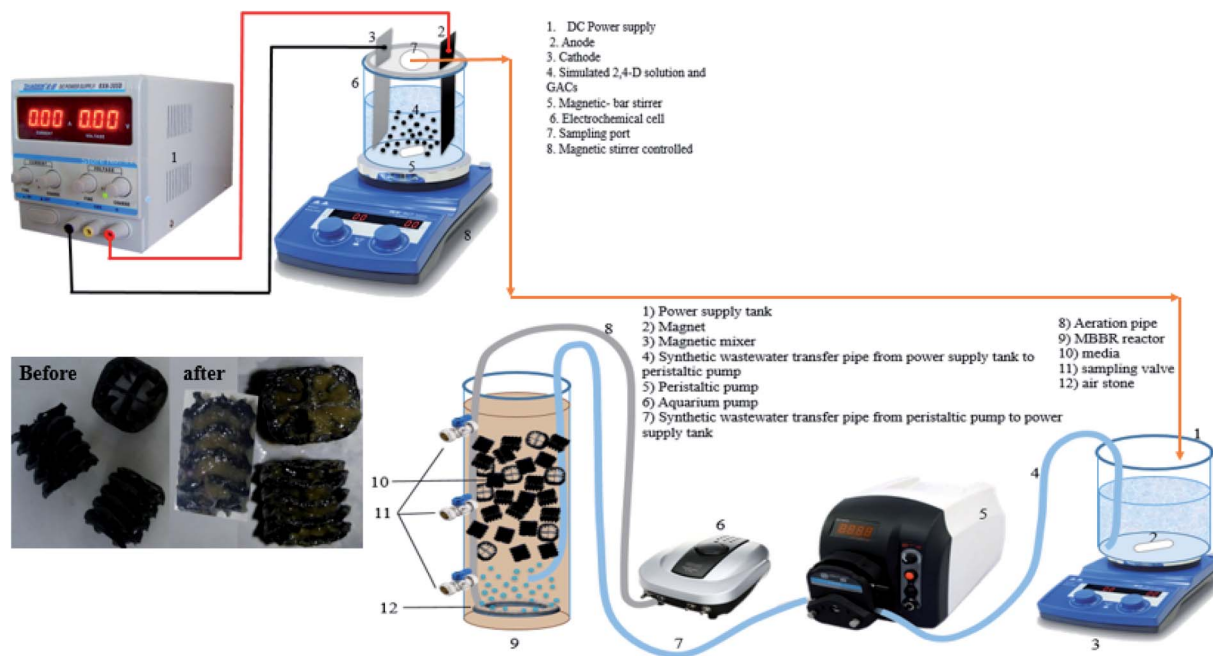
Fig. 1 Schematic of reactor used in this study.
