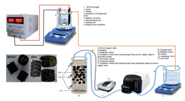
Fig. 1 Schematic of reactor used in this study.
