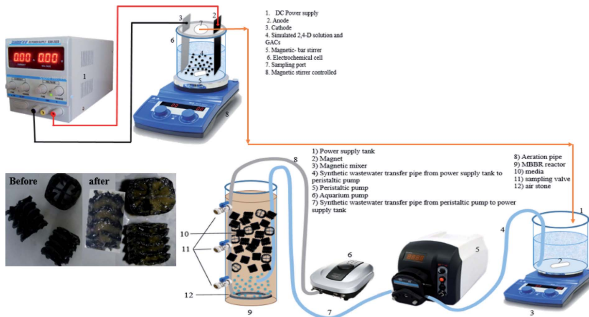
Fig. 1 Schematic of reactor used in this study.
