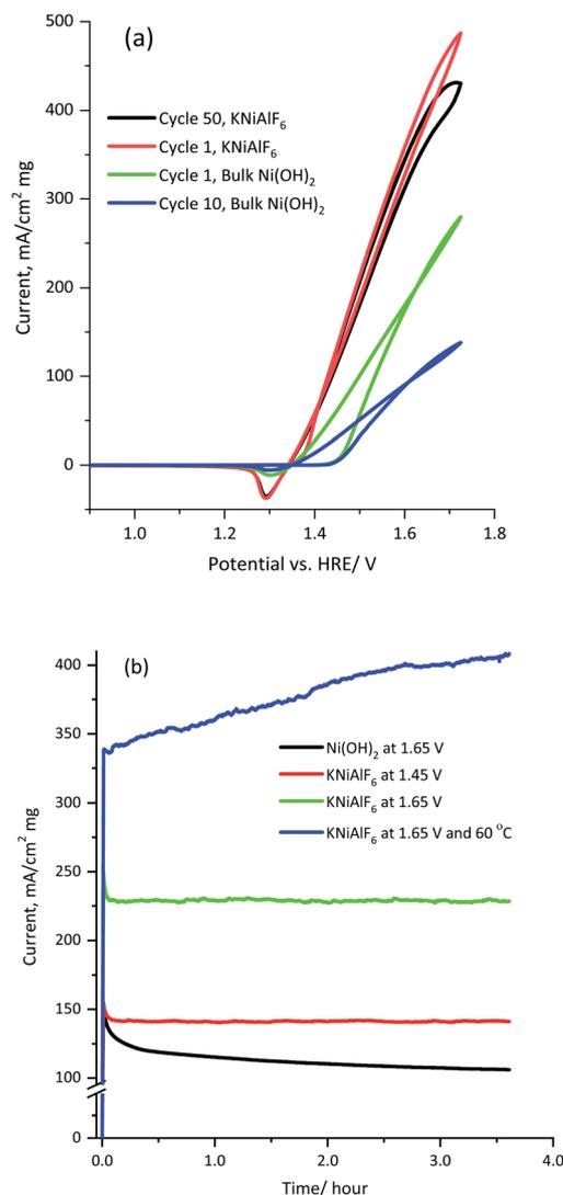
Fig. 8 (a) Multicycles voltammograms obtained for 100  $\mu\text{g}$  of the  $\text{KNiAlF}_6$  and bulk catalysts recorded at 50  $\text{mV s}^{-1}$  in 1.0 M KOH solution containing 0.33 M urea and (b) the corresponding chronoamperometry recorded at various applied voltages (1.45 and 1.65 V vs. HRE/V) and temperature (25 and 60  $^{\circ}\text{C}$ ).
