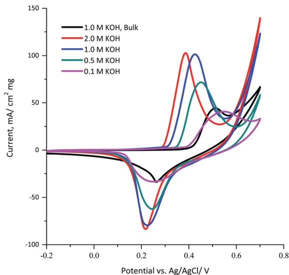
Fig. 5 Cyclic voltammograms obtained for 100 μg of the KNiAlF<sub>6</sub> and bulk Ni(OH)<sub>2</sub> catalysts recorded at a scan rate of 50 mV s<sup>-1</sup> in various concentrations of KOH solution (0.1, 0.5, 1.0, and 2.0 M).
