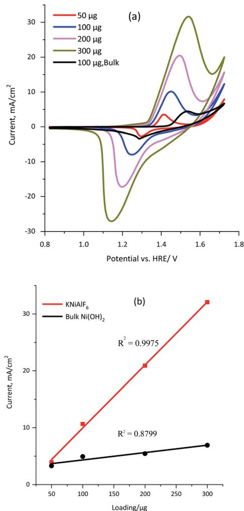
Fig. 4 (a) Cyclic voltammograms obtained for the KNiAlF<sub>6</sub> catalyst using various loadings of 50, 100, 200, and 300 μg in 1.0 M KOH solution and 100 μg of the bulk Ni(OH)<sub>2</sub> catalyst (black line) recorded at a scan rate of 50 mV s<sup>-1</sup>. (b) Relationship between the catalyst loading and current observed for both the KNiAlF<sub>6</sub> and bulk Ni(OH)<sub>2</sub> catalysts.
