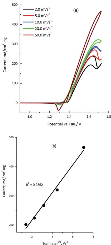
Fig. 7 (a) Cyclic voltammograms obtained for 100  $\mu\text{g}$  of the  $\text{KNiAlF}_6$  catalyst in 1.0 M KOH solution containing 0.33 M urea recorded at various scan rates (2.0, 5.0, 10.0, 20.0, and 50.0  $\text{mV s}^{-1}$ ). (b) The plot of current vs. square root of the scan rate.
