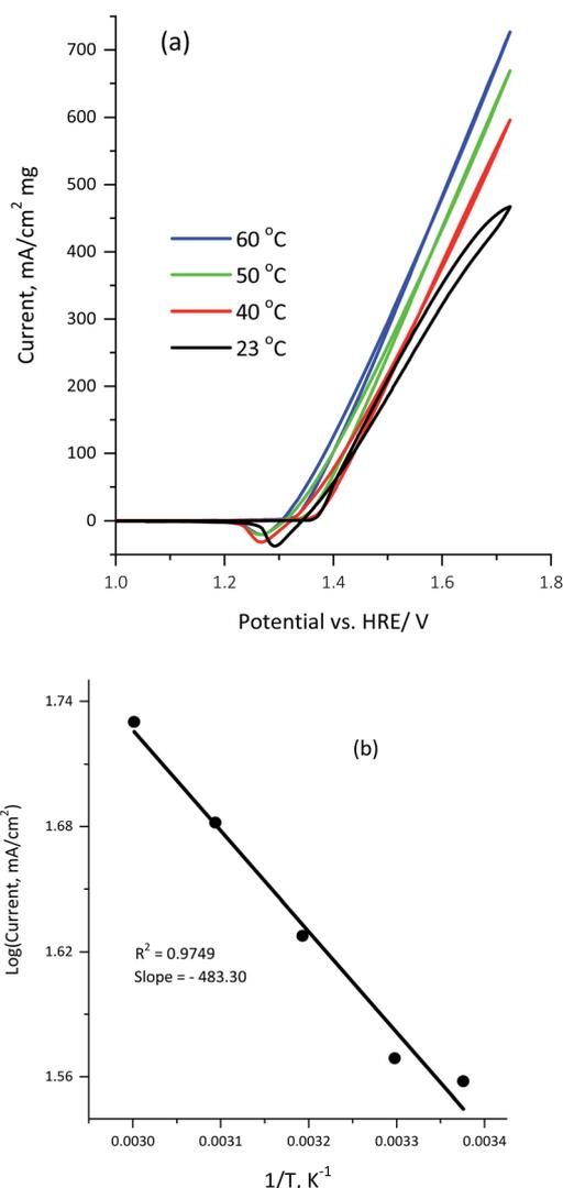
Fig. 9 (a) Cyclic voltammograms obtained for 100  $\mu$ g of the KNiAlF<sub>6</sub> catalyst recorded in 0.33 M urea at various temperatures (23, 30, 40, 50, and 60 °C). (b) The plot of the logarithm rate vs. the reciprocal of the absolute temperature.
