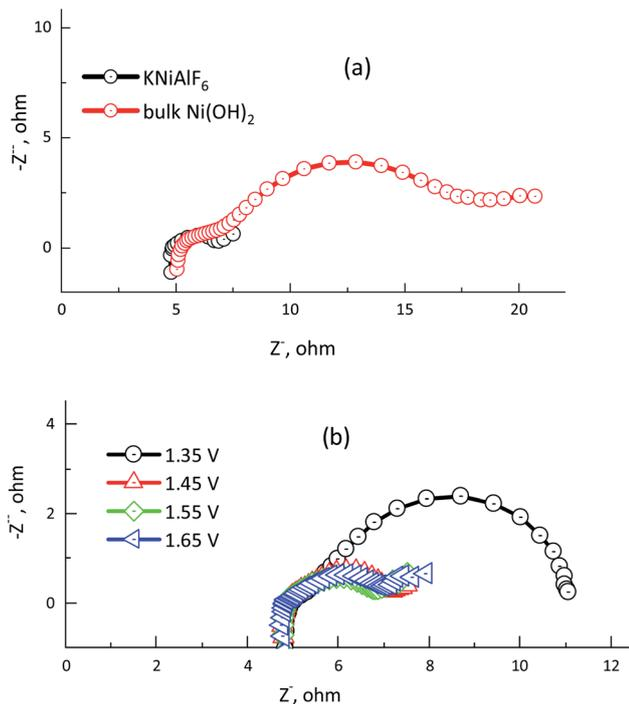
Fig. 10 (a) Nyquist plot obtained for 100  $\mu\text{g}$  of the KNiAlF<sub>6</sub> and bulk Ni(OH)<sub>2</sub> catalysts recorded at 1.65 V vs. HRE. (b) Nyquist plot obtained for 100  $\mu\text{g}$  of the KNiAlF<sub>6</sub> catalyst recorded at various potentials: 1.35, 1.45, 1.55, and 1.65 V vs. HRE in 1.0 M KOH solution containing 0.33 M urea.
