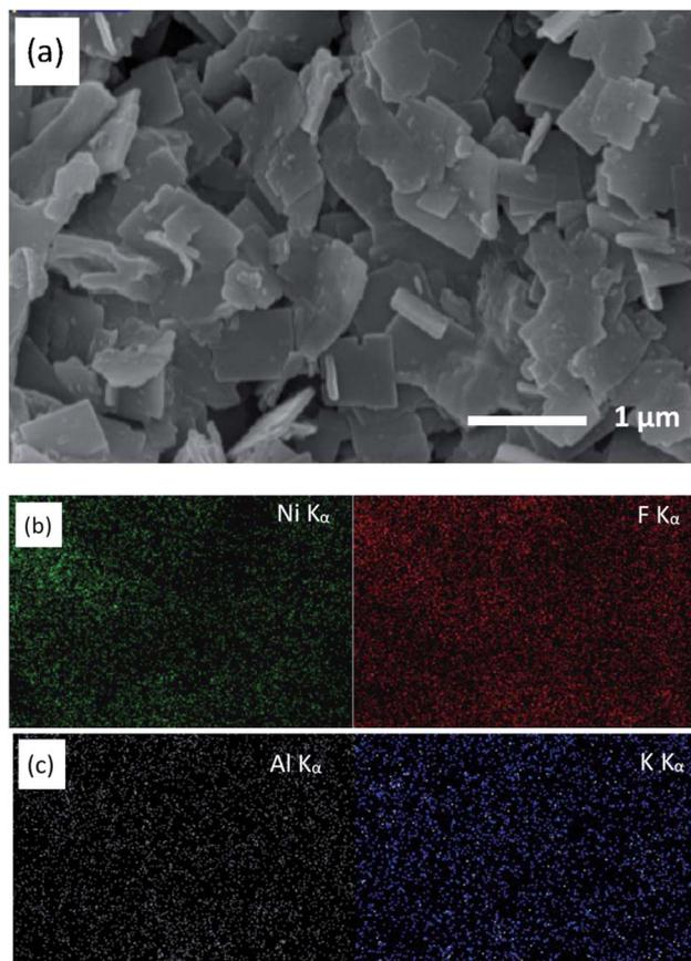
Fig. 3 (a) SEM image and (b and c) corresponding X-ray elemental mapping of the KNiAlF<sub>6</sub> catalyst.
