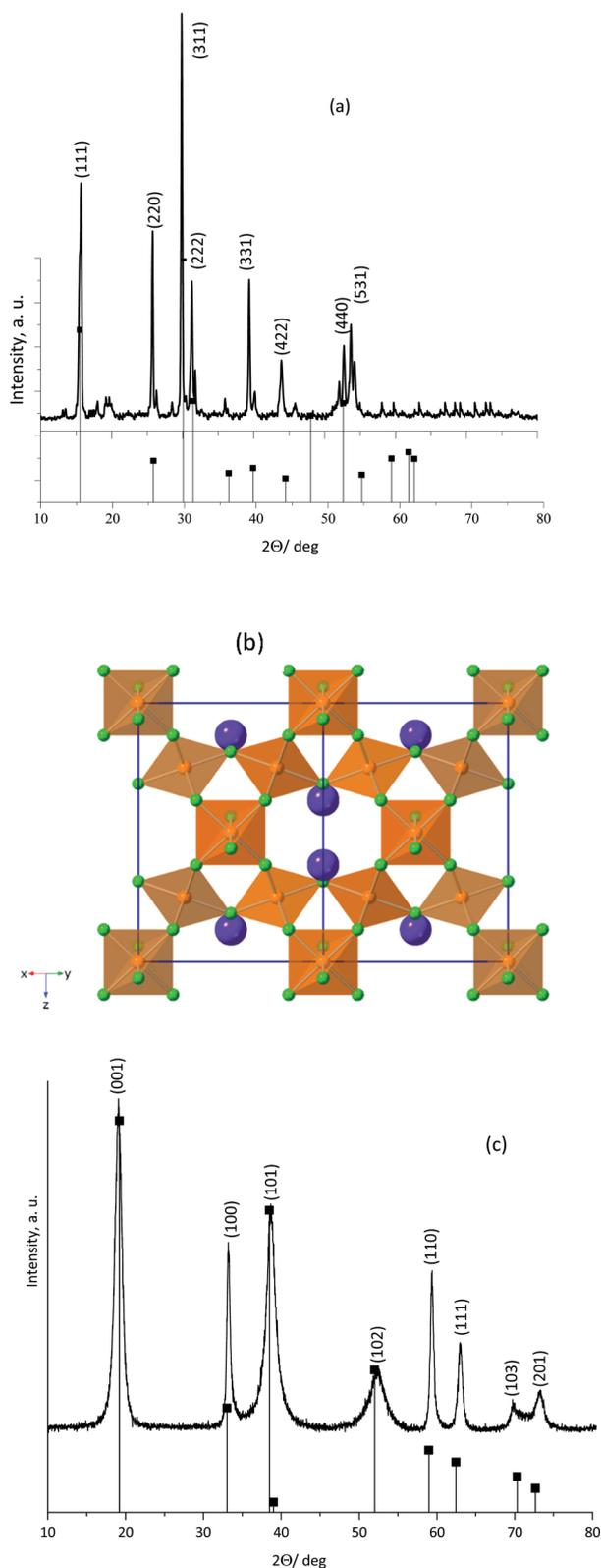
Fig. 1 (a) Powder X-ray diffraction (PXRD) patterns obtained for the (a)  $\text{KNiAlF}_6$ , (b) the structure of  $\text{KNiAlF}_6$ , the  $(\text{Ni}_{0.5}\text{Al}_{0.5})\text{F}_6$  octahedra are shown in orange,  $\text{K}^+$  cations are large purple spheres and  $\text{F}^-$  ions are green and (c) PXRD pattern of bulk  $\text{Ni}(\text{OH})_2$  catalysts.
