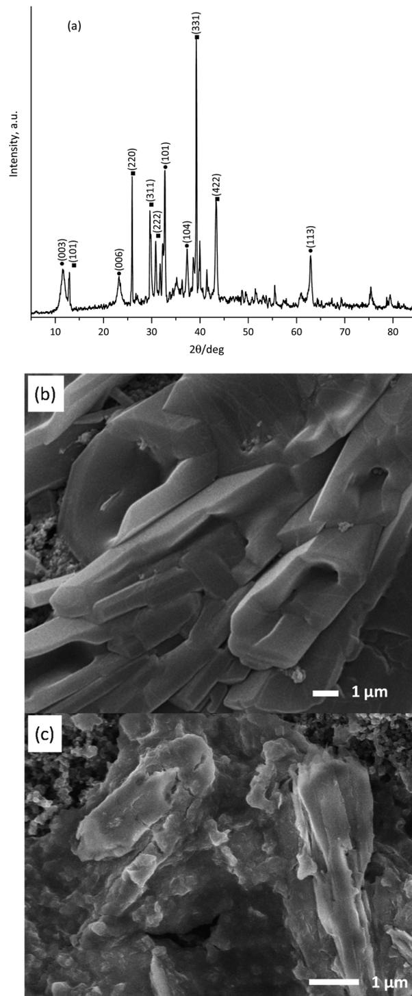
Fig. 11 (a) Powder X-ray diffraction pattern obtained for the  $\text{KNiAlF}_6$  catalyst after being used in the electrolysis in 1.0 M KOH solution containing 0.33 M urea performed at 1.65 V vs. HRE for 3 hours, (b) SEM images of the  $\text{KNiAlF}_6$  catalyst after being used in the electrolysis of a 1.0 M KOH solution containing 0.33 M urea performed at 1.65 V vs. HRE for 3 h at 25 °C and (c) at 60 °C.
