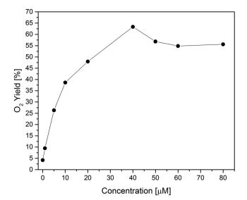
Fig. 4 Photocatalytic oxygen yield vs. WOC concentration for Co(1)
