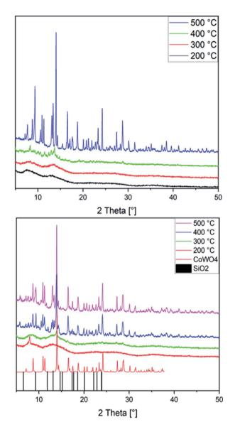
Fig. 2 PXRD patterns of the CoNiX00 (top) and CoWX00 (bottom) series annealed at 200  $^{\circ}$ C (black) up to 500  $^{\circ}$ C (purple; CoWO<sub>4</sub>: CCDC-619251, SiO<sub>2</sub>: PDF No. 12-0711).
