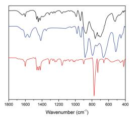
Fig. 5 FT-IR spectra of the Co(1)-POM-PS complex (black), pristine Co(1) (blue) and  $[Ru(bpy)_{\overline{1}}]Cl_2$  (red).
