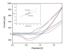
Fig. 8 Cyclic voltammograms of CoW300 (black); CoWO $_4$  (red); RuO $_2$  (blue) and reference FTO (dotted) in 0.1 M borate buffer pH 8 (scan rate: 20 mV s $^{-1}$ ); inset: Tafel plot of CoW300 (black) and CoWO $_4$  (red).
