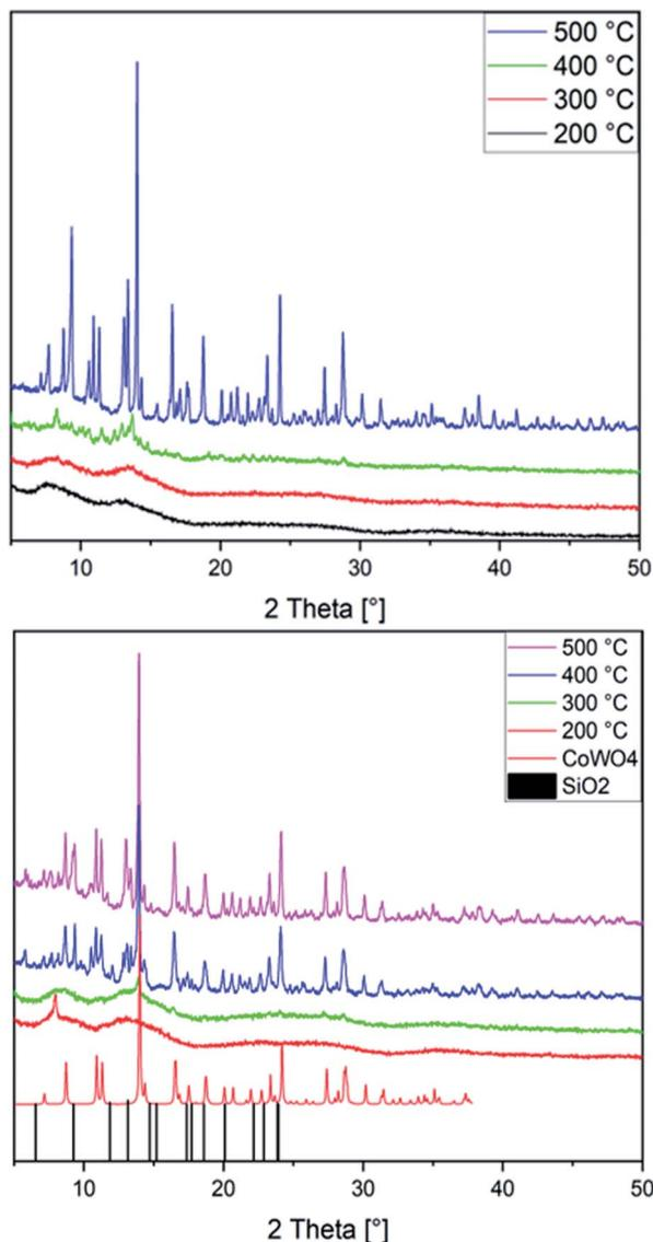
Fig. 2 PXRD patterns of the CoNiX00 (top) and CoWX00 (bottom) series annealed at 200 °C (black) up to 500 °C (purple; CoWO<sub>4</sub>: CCDC-619251, SiO<sub>2</sub>: PDF No. 12-0711).
