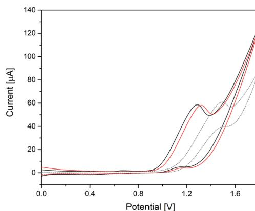
Fig. 6 Cyclic voltammograms of 50  $\mu\text{M}$  **Co(1)** (black) and 50  $\mu\text{M}$  **CoNi(2)** (red) in 0.1 M borate buffer pH 8 and blank measurements (grey, dashed; V vs. Ag/AgCl, scan rate: 20  $\text{mV s}^{-1}$ , 3<sup>rd</sup> scan is shown).
