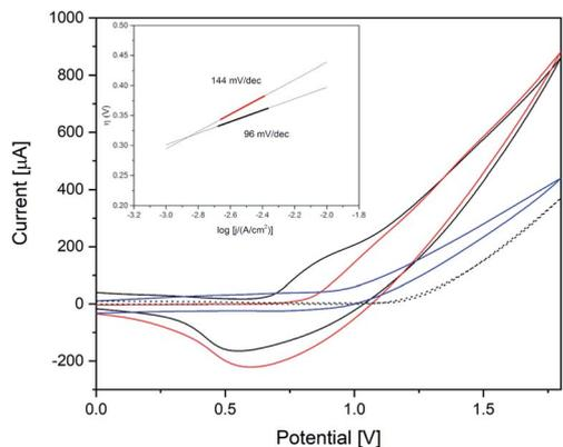
Fig. 8 Cyclic voltammograms of CoW300 (black); CoWO<sub>4</sub> (red); RuO<sub>2</sub> (blue) and reference FTO (dotted) in 0.1 M borate buffer pH 8 (scan rate: 20 mV s<sup>-1</sup>); inset: Tafel plot of CoW300 (black) and CoWO<sub>4</sub> (red).
