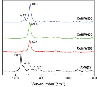
Fig. 3 Raman spectra of Co(1) together with the CoW300/400/500 series (top; black/red/green/blue) and of compound CoNi(2) with the CoNiW300/400/500 series (bottom; black/red/green/blue).
