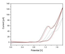
Fig. 6 Cyclic voltammograms of 50  $\mu$ M Co(1) (black) and 50  $\mu$ M CoNi(2) (red) in 0.1 M borate buffer pH 8 and blank measurements (grey, dashed; V vs. Ag/AgCl, scan rate: 20 mV s<sup>-1</sup>, 3<sup>rd</sup> scan is shown).
