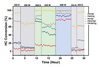
Fig. 9 Cyclic stability test results for the prepared catalysts under dry and wet (12 vol%  $H_2O$ ) conditions. Feed composition: 1.0 vol%  $CH_4$ , 1000 ppm  $C_2H_4$ , 22%  $O_2$  diluted with nitrogen at a GHSV of 80 000 mL  $q_{\rm cat}^{-1}$   $h^{-1}$ .
