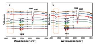
Fig. 7 DRIFT spectra for (a) Pd/YSZ and (b) Pd/ZrO $_2$ . The analyses were performed at a flow of 2% CH $_4$ /N $_2$  and O $_2$  (20 vol%) at temperatures of 250 °C (i–iii), 350 °C (iv–vi), and 550 °C (vii–ix) in a continuous flow (33.33 mL min $^{-1}$ ) heated cell.
