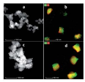
Fig. 5 STEM and EDX elemental mapping (a and b) PdPt/YSZ, (c and d) PdPt/ZrO<sub>2</sub>.
