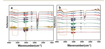
Fig. 8 DRIFT spectra for (a) Pd-Pt/YSZ and (b) PdPt/ZrO<sub>2</sub>. The analyses were carried out at a flow (33.33 mL min<sup>-1</sup>) of 2% CH<sub>4</sub>/N<sub>2</sub> and O<sub>2</sub> (20 vol%) at temperatures of 250 °C (i, ii, iii), 350 °C (iv, v, vi), and 550 °C (vii, viii, ix) in a heated cell.
