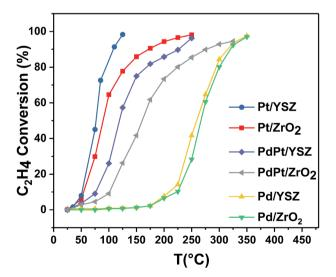
Fig. 2 Light-off temperature profile of  $C_2H_4$  oxidation over the synthesized catalysts (mass of catalyst: 0.025 g; total flow rate: 33.33 mL min<sup>-1</sup>; 1000 ppm  $C_2H_4/22\%$   $O_2$  in balance Ar; GHSV: 80 000 mL  $g_{cat}^{-1}$  h<sup>-1</sup>).
