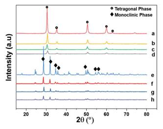
Fig. 4 X-ray diffraction patterns of supports and pristine catalysts calcined at 600 °C for 3 h in air. (a) YSZ (b) Pd/YSZ (c) Pt/YSZ (d) PdPt/YSZ (e) ZrO<sub>2</sub> (f) Pd/ZrO<sub>2</sub> (g) PdPt/ZrO<sub>2</sub> and (h) Pt/ZrO<sub>2</sub>.
