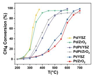
Fig. 1 Light-off temperature profiles of CH $_4$  oxidation over the synthesized catalysts (mass of catalyst: 0.025 g; total flow rate: 33.33 mL min $^{-1}$ ; 1 volume% CH $_4$  in 20% O $_2$ , balance N $_2$ ; GHSV: 80 000 mL  $_{Cat}^{-1}$  h $^{-1}$ ).
