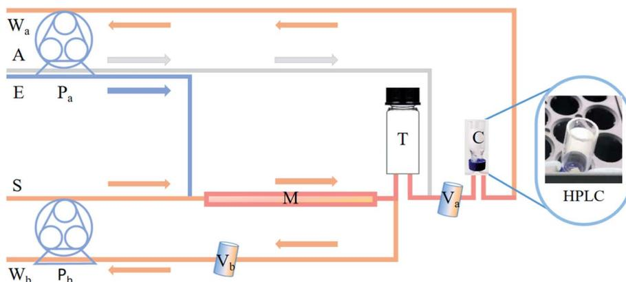
Fig. 1 Self-designed SPE-HPLC system. Air stream (A), HPLC cup (C), eluent stream (E), extraction microcolumn (M), peristaltic pump a (P<sub>a</sub>), peristaltic pump b (P<sub>b</sub>), sample stream (S), tube (T), valve a (V<sub>a</sub>), valve b (V<sub>b</sub>), liquid waste (W<sub>a</sub>), liquid waste (W<sub>b</sub>).
