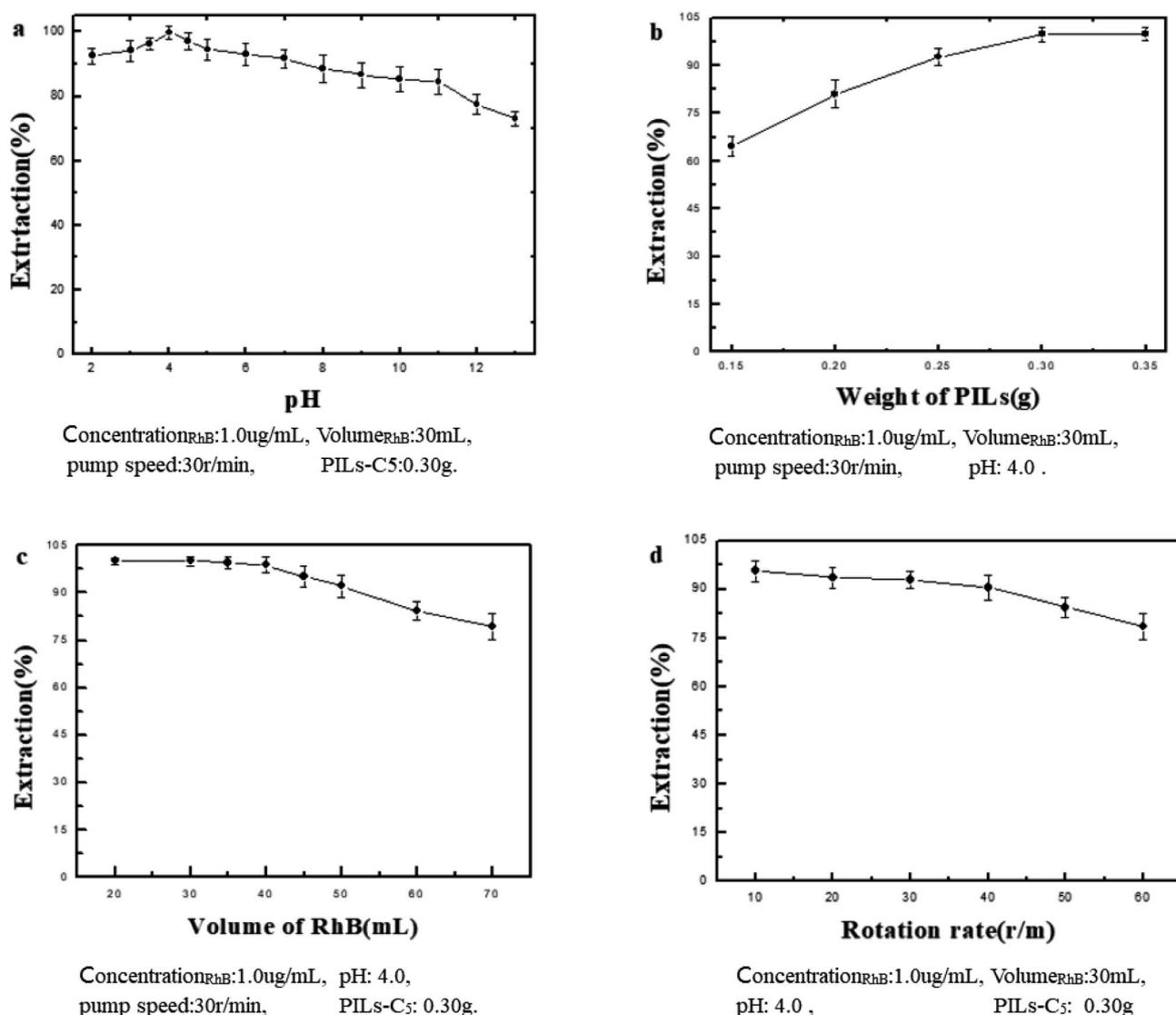
Fig. 4 Optimization of extraction parameters by SFED.
