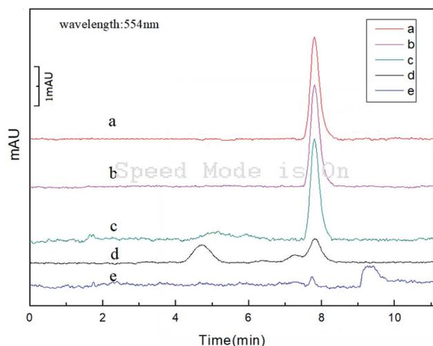
Fig. 7 Analysis of real samples. (a) RhB ( $0.6 \mu\text{g mL}^{-1}$ ); (b) shampoo (after extraction); (c) lipstick (after extraction); (d) shampoo (before extraction); (e) lipstick (before extraction).
