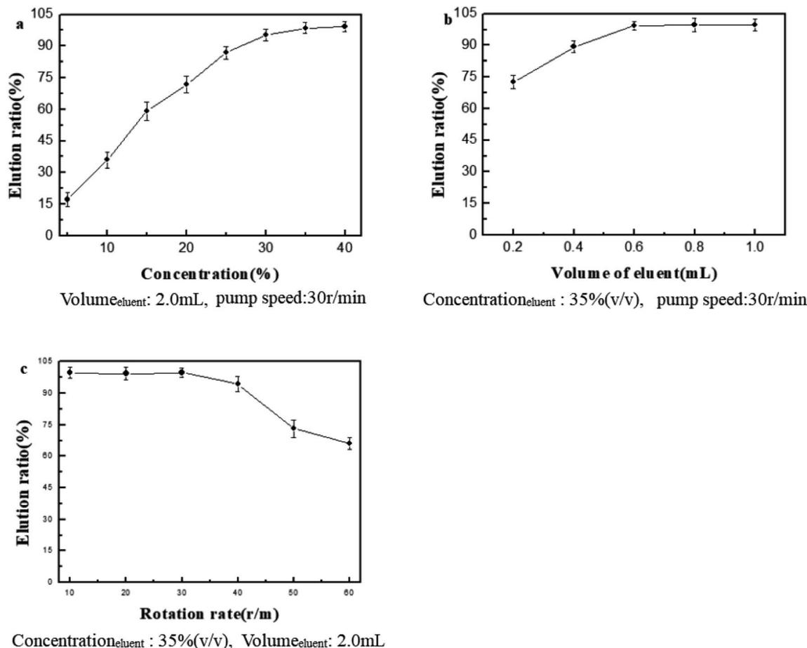
Fig. 5 Optimization of elution parameters by SFED.
