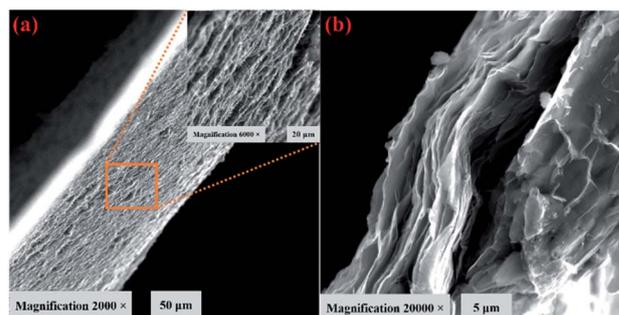
Fig. 2 FE-SEM images of (a) cross sectional views of BN/GrP (inset) at low and (b) high magnifications.
