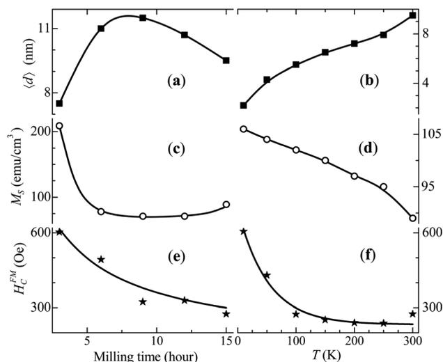
Fig. 6 Parameters estimated from the magnetization hysteresis loops' simulations for different milling times of  $\text{Co}_{50}\text{Te}_{50}$  (left panels) at 300 K and for different measurement temperatures (right panels) for the 15 hour milled sample. Panels (a) and (b): the mean size of the SPM part of each sample; (c) and (d): total saturation magnetization; (e) and (f): coercive field of the respective ferromagnetic part. The lines are merely guides for the eye.
