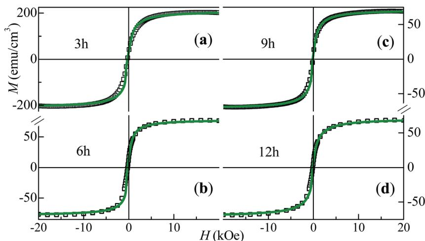
Fig. 5 Symbols: descending branches of the  $M \times H$  loops obtained at 300 K via VSM measurements for  $\text{Co}_{50}\text{Te}_{50}$  with different milling times; the lines are the respective fitting curves.
