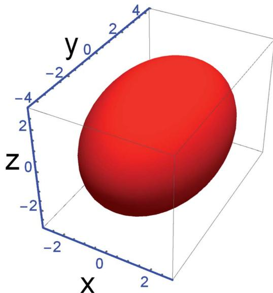
Fig. 2 Crystallite size anisotropy modeled with a triaxial ellipsoid. Values are  $r_x = r_z = 2.855$  nm and  $r_y = 4.310$  nm.  $R$ -values:  $R_{wp}$  of 2.78% ( $R_p$  2.11%) and GoF 1.702.
