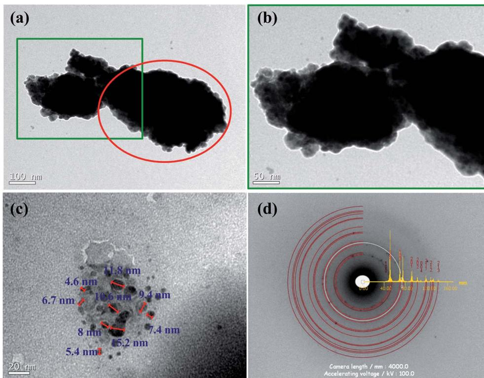
Fig. 3 (a) TEM 100 kV image of the  $\text{Co}_{50}\text{Te}_{50}$  milled for 15 h. (b) Magnified image corresponding to the green square. (c) Another picture from the sample showing the crystallite sizes. (d) SAED measurements modeled with JEMS. The white ring was fitted for the Co/Fe phase, and the red rings represent the  $\beta$ -CoTe. The  $hkl$ s of each peak are above them.
