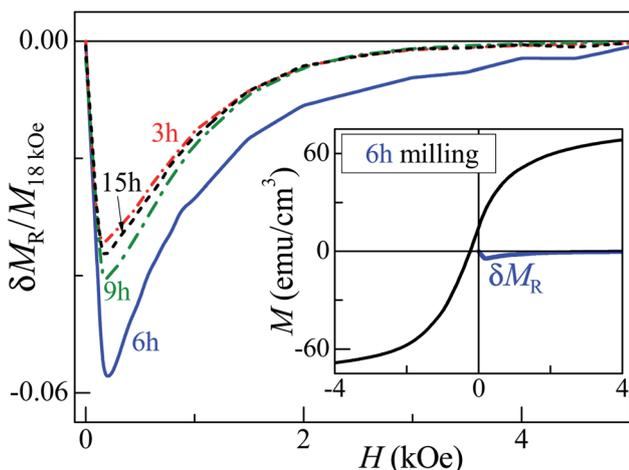
Fig. 7  $\delta M_R$  interaction plots, obtained from recoil loops with recoil fields equal to the respective coercive field value at 300 K, of  $\text{Co}_{50}\text{Te}_{50}$  samples for different ball-milling times. The inset gives the  $\delta M_R$  plot with the greatest amplitude together with the descending branch of the corresponding major loop.
