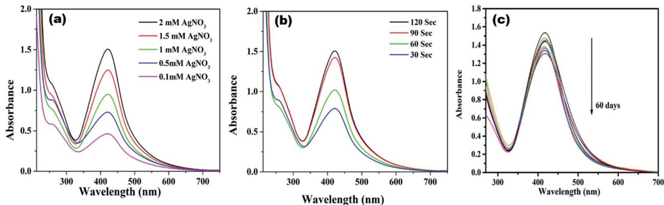
Fig. 2 UV-vis absorption spectra of AgNPs/NCDs nanocomposite synthesized at (a) different concentration of  $\text{AgNO}_3$ , and (b) different microwave irradiation time; (c) UV-vis spectra of AgNPs/NCDs depicting their stability for 2 months.
