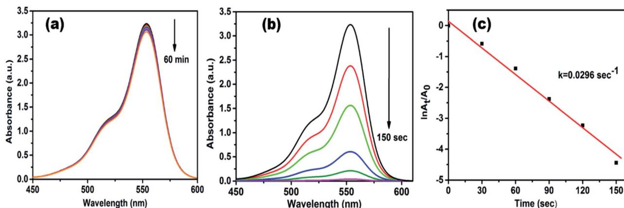
Fig. 7 UV-vis absorption spectra of (a) catalytic reduction of RhB in the presence of  $\text{NaBH}_4$  and in the absence of catalyst; (b) time-dependent absorption spectra of RhB in the existence of both  $\text{NaBH}_4$  and AgNPs/NCDs; (c) plot of  $\ln(A_t/A_0)$  against time for reduction of RhB dye.
