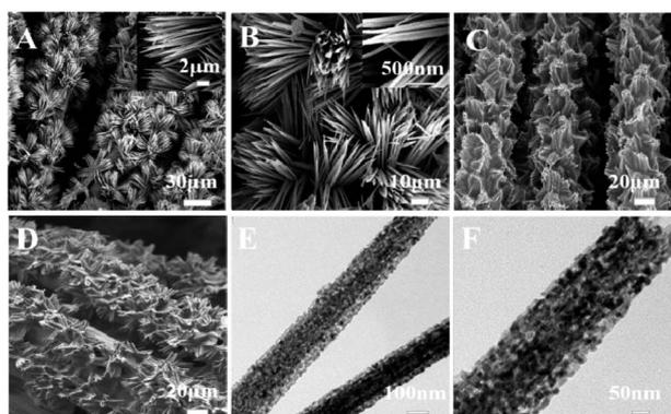
Fig. 1 (A) SEM images of CoN precursor, (B) CoN/CC (the inset displaying the corresponding SEM image at high magnification), (C) MIP/Ru(bpy)<sub>3</sub><sup>2+</sup>/Nafion/CoN/CC before elution, (D) NIP/Ru(bpy)<sub>3</sub><sup>2+</sup>/Nafion/CoN/CC before elution, (E) low-magnification TEM image of CoN/CC, (F) high-magnification TEM image of CoN/CC.
