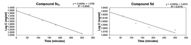
Fig. 6 Graphical representation of first-order kinetic isomerization of the E/Z diastereomers for representative compounds 5c<sub>2</sub> and 5d
