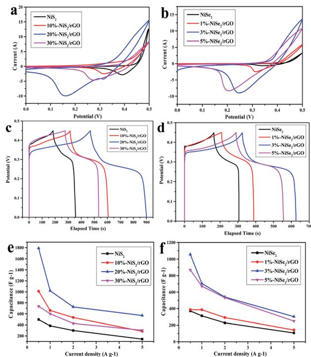
Fig. 4 (a) and (b) CV curves of the four electrodes at a scan rate of  $10 \text{ mV s}^{-1}$ ; (c) and (d) GCD curves of the four electrodes at a current density of  $1 \text{ A g}^{-1}$ ; (e) and (f) specific capacitances of the four electrodes at various current densities.
