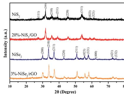
Fig. 2 XRD patterns of the synthesized products.
