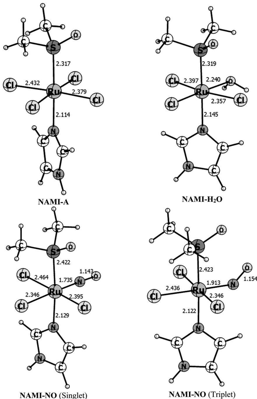
Fig. 1 Gas phase B3LYP/def2-TZVP optimized parameters for the complexes NAMI-A, NAMI-H<sub>2</sub>O and NAMI-NO in the singlet and triplet states. Bond distances in Å and bond angles in degrees.
