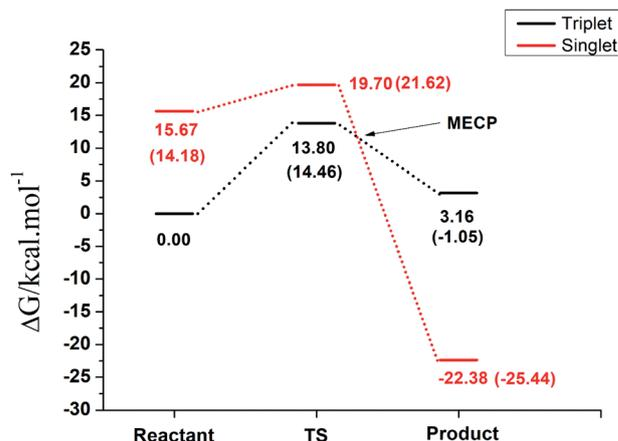
**Fig. 6** Overall energy profile in aqueous solution, computed at the B3LYP/def2-TZVP(SMD) for the NO–H<sub>2</sub>O exchange reaction [RuCl<sub>3</sub>(-H<sub>2</sub>O)(Im)(DMSO)] + NO → [RuCl<sub>3</sub>(NO)(Im)(DMSO)] + H<sub>2</sub>O, in the singlet and triplet spin states. Values in parenthesis were obtained in aqueous solution.
