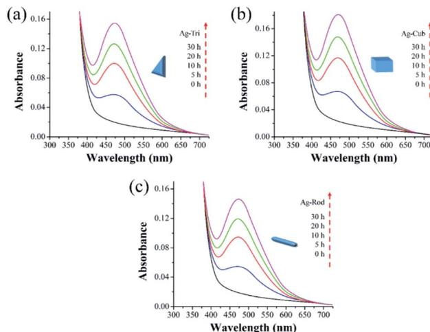
Fig. 7 Superoxide ( $O_2^{\cdot-}$ ) generation kinetics of anisotropic silver nanoparticles under UV irradiation. The spectra generated at 470 nm indicated by the reduction of 100  $\mu\text{M}$  XTT (a)  $O_2^{\cdot-}$  generation by Ag-Tri (b)  $O_2^{\cdot-}$  by Ag-Cub (c)  $O_2^{\cdot-}$  generation by Ag-Rod.
