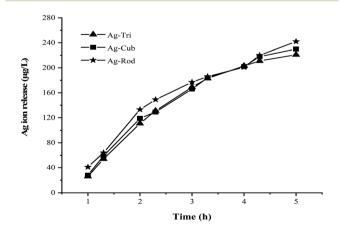
Fig. 9 Silver ion release profile of anisotropic silver nanoparticles with UV irradiation.
