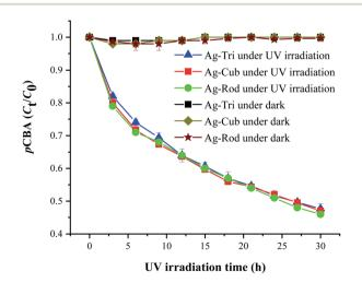
Fig. 8  $\,^{\circ}$ OH generation kinetics under UV irradiation of the aqueous suspension of anisotropic AgNPs, as shown by the degradation of 20  $\mu$ M  $\rho$ CBA.
