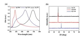
Fig. 1 (a) Illustrated the UV spectra of anisotropic AgNP with their characteristic peaks at  $\sim\!\!360$  and 380 nm for Ag-Rod 420 and  $\sim\!\!565$  nm for Ag-Cub and the peaks at  $\sim\!\!520$  nm and  $\sim\!\!690$  nm for Ag-Tri. (b) XRD spectra of anisotropic AgNP of Ag-Tri, Ag-Rod and Ag-Cub respectively.
