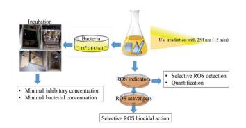
Fig. 3 Schematic diagram of the methodological workflow illustrating anisotropic AgNP individual shape UV irradiation to MIC, MBC, and ROS generation and quantification steps.
