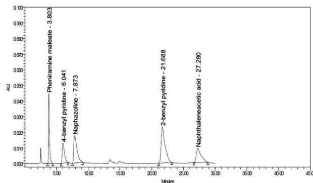
Fig. 2 HPLC chromatograms of NPZ ( $35.00 \mu\text{g mL}^{-1}$ ), PHN ( $90.00 \mu\text{g mL}^{-1}$ ) and three of their selected impurities; NPZ impurity B ( $35.00 \mu\text{g mL}^{-1}$ ), PHN impurity A ( $50.00 \mu\text{g mL}^{-1}$ ) and PHN impurity B ( $90.00 \mu\text{g mL}^{-1}$ ) using a hypersil ODS column (5 mm, 250–4.6 mm i.d.), mobile phase of pH 6.0 phosphate buffer: acetonitrile (70 : 30, by volume), flow rate of  $1.0 \text{ mL min}^{-1}$  and detection at 260 nm.
