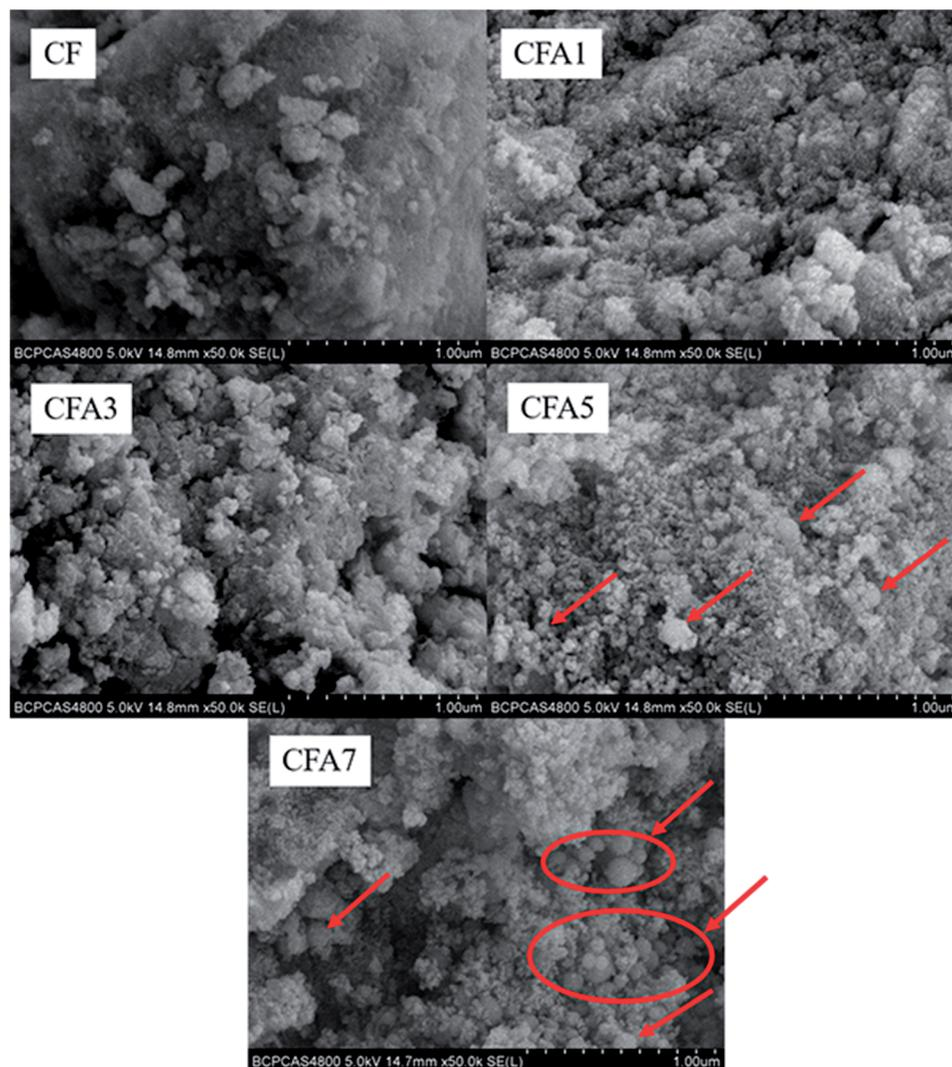
Fig. 3 SEM images of Al/copper ferrites MICs.
