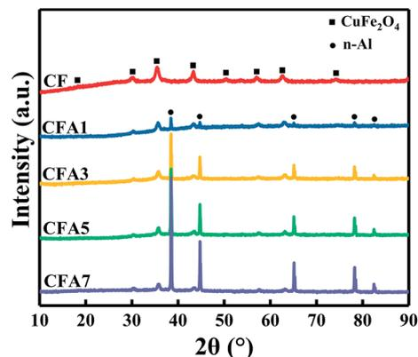
Fig. 2 X-ray diffraction patterns of Al/copper ferrites MICs.
