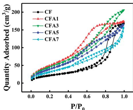
Fig. 4 Nitrogen adsorption–desorption isotherms of Al/copper ferrites MICs.
