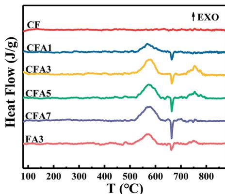
Fig. 6 DSC curves of Al/copper ferrites MICs.
