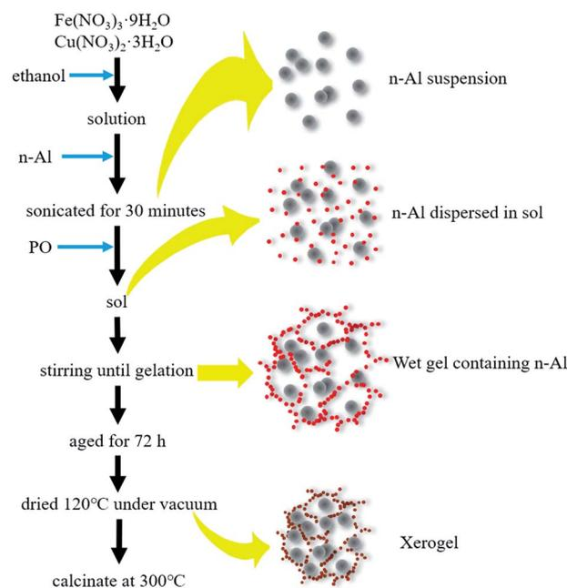
Fig. 1 Preparing process of Al/copper ferrites MICs.
