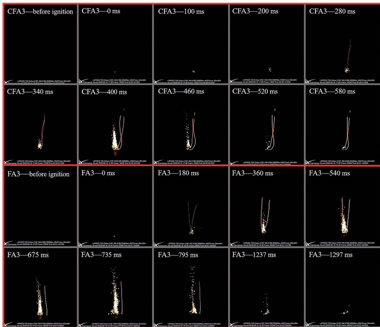
Fig. 8 High-speed photographs of Al/copper ferrites and Al/Fe<sub>2</sub>O<sub>3</sub> MICs.
