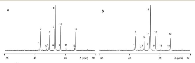
Fig. 4 The <sup>13</sup>C NMR spectra of EPDM rubber: the pristine (a) and modified (b) samples. The modified sample synthesised using the VOCl<sub>3</sub>/EASC/ HCPX catalytic system.
