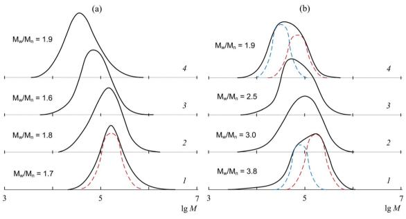
Fig. 5 MWD of the ethylene-propylene copolymer. Copolymerisation conditions: the VOCl3-EASC (a) and VOCl3-EASC-HCPX (b) catalytic systems; copolymerisation temperatures: 20 (1), 30 (2), 40 (3), and 50 (4) °C; P = 0.6 MPa;  $\tau = 60$  min; the Al/V molar ratio = 50.
