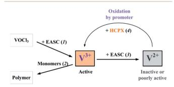
**Scheme 2** Simplified reaction pathways involved in ethylene and propylene copolymerisation performed with vanadium catalyst system and hexachloro-*p*-xylene.
