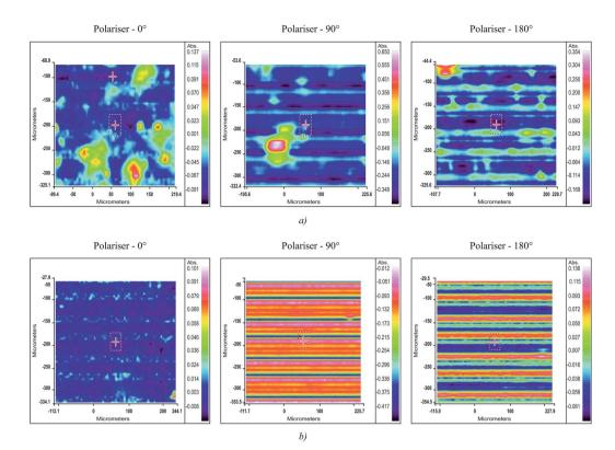
Fig. 3 The IR images of the copolymer samples. (a) Copolymer 1 (sample 1) synthesised over the VOCl3-EASC catalytic system; (b) the copolymer (sample 4) synthesised using the VOCl<sub>3</sub>/EASC/HCPX catalytic system.
