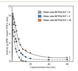
Fig. 2 Changes in activity of the VOCl<sub>3</sub>–EASC–HCPX catalytic system as a function of ethylene–propylene copolymerisation duration. The  $C_6H_4(CCl_3)_2/VOCl_3$  molar ratio: 1–0; 2–4; 3–10. Copolymerisation conditions:  $T_p=30~^{\circ}C$ , P=0.6 MPa,  $\tau=60$  min; Al/V molar ratio = 50.
