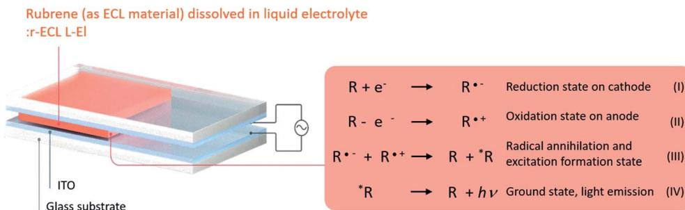
Fig. 2 Illustrated description of the prepared r-ECL L-EI cell structure, and ECL mechanism which occurs due to the electrochemical redox reaction under the applied square-wave AC voltage.
