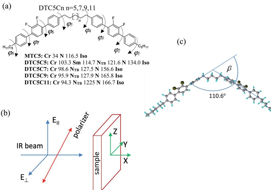
Fig. 1 2',3'-Difluoro-4,4''-dipentyl-*p*-terphenyl dimers (DTC5Cn) ( $n = 5, 7, 9, 11$ ). (a) Transition temperature and molecular structure of DTC5Cn. (b) Schematic of polarized infrared transmission technique at a normal incidence of light. (c) Simulated structure of the helical conformer of DTC5C5 molecule.  $\beta$  –angle, that *para*-axes of rigid cores make with each other.
