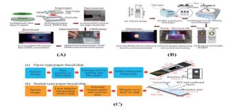
Fig. 9 (A) Schematic illustration of microfluidic paper-based/PMMA chip and schematic illustration of associated SO<sub>2</sub> con-centration detection procedure. (B) Schematic illustration showing fabrication procedure for microfluidic paper-based chip and associated benzoic acid concentration detection process. (C) Main steps in the manufacturing process: (a) open-type chip and (b) sealed-type chip.
