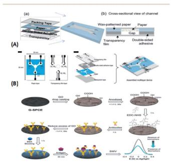
Fig. 15 (A) Assembly and flow characteristics of microfluidic paperbased analytical devices (µPADs). (a) Schematic of fast-flow µPAD assembly. (b) Cross-sectional view of channel of fast flow µPADs. (B) Design and fabrication of the multiplexed ePADs and step-by-step preparation of the electrochemical immunosensor and detection of the antigen/biomarker on the sensor
