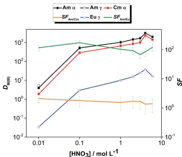
Fig. 3 Distribution ratios of Am(III), Cm(III) and Eu(III) as a function of the aqueous feed acidity. Org.: 0.01 mol L<sup>-1</sup> CyMe<sub>4</sub>BTPhen in [A336][NO<sub>3</sub>], Aq.: 0.01–6 mol L<sup>-1</sup> HNO<sub>3</sub>, Ln(III) = 10<sup>-5</sup> mol L<sup>-1</sup>, T = 30 °C, shaking at 2400 rpm for 12 h.
