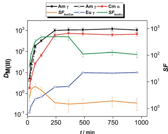
Fig. 2 Distribution ratios of Am(III), Cm(III) and Eu(III) and the corresponding separation factors as a function of the equilibration time. Org.:  $0.01\ \text{mol L}^{-1}$  CyMe<sub>4</sub>BTPPhen in [A336][NO<sub>3</sub>], Aq.:  $1\ \text{mol L}^{-1}$  HNO<sub>3</sub>, Ln(III) =  $10^{-5}\ \text{mol L}^{-1}$ ;  $T = 30\ ^\circ\text{C}$ , shaking at 2400 rpm.
