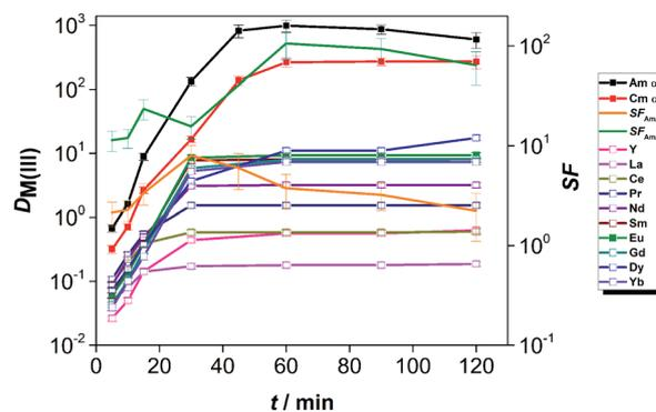
Fig. 5 Distribution ratios of An(III) and Ln(III) as a function of equilibration time. Org.: 0.01 mol L<sup>-1</sup> CyMe<sub>4</sub>BTPhen + 0.005 mol L<sup>-1</sup> TODGA in a diluent mixture composed of 70 vol% [A336][NO<sub>3</sub>] and 30 vol% 1-octanol; Aq.: 1 mol L<sup>-1</sup> HNO<sub>3</sub>, [Ln(III)] (La–Dy, Yb, Y) = 10<sup>-5</sup> mol L<sup>-1</sup>; spiked with tracers of <sup>241</sup>Am, <sup>244</sup>Cm and <sup>152</sup>Eu. T = 30 °C, shaking at 2400 rpm.
