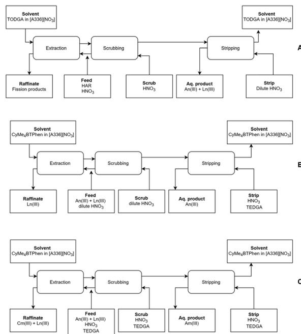
Fig. 7 Preliminary flow sheets for the separation of Am(III) + Cm(III) (A + B) or separation of Am(III)-only (A + C) from a highly active raffinate feed solution using a [A336][NO<sub>3</sub>]-based process. For flow sheet B, TODGA (as phase transfer catalyst) and 1-octanol (as co-diluent) can be added to the solvent to improve kinetics. For flow sheet C, 1-octanol (as co-diluent) can be added to the solvent to improve kinetics.
