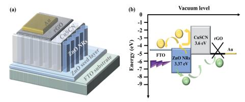
Fig. 6 (a) Schematic and (b) energy band of the FTO/Zn NR/CuSCN/rGO/Au junction
