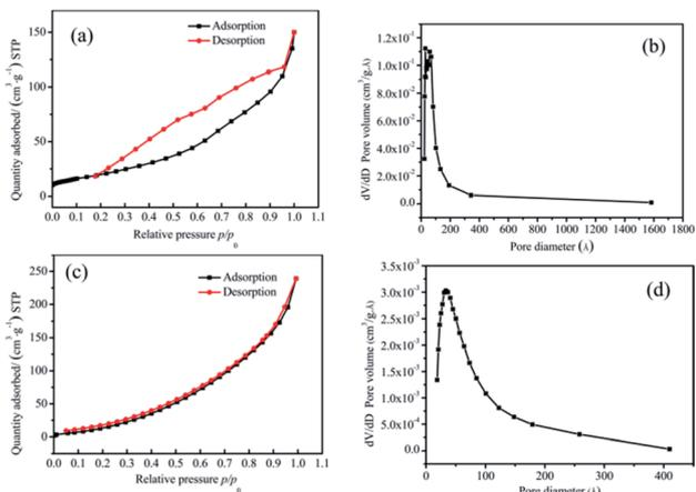
Fig. 4 (a) and (b) The nitrogen adsorption–desorption isotherms and pore size distribution of pure  $\text{Co}_3\text{O}_4$  nano-fibers, respectively. (c) and (d) The nitrogen adsorption–desorption isotherms and pore size distribution of the 20 : 2 sample.
