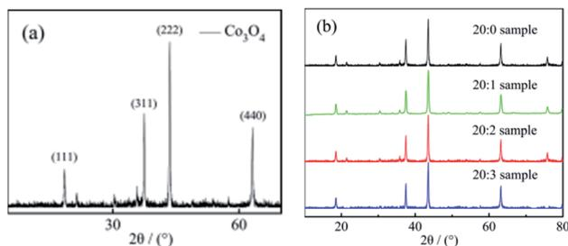
Fig. 1 (a) The XRD test results of the pure  $\text{Co}_3\text{O}_4$  working electrode sample; (b) the XRD test results of the  $\text{Co}_3\text{O}_4$  composite working electrode doped with  $\text{Mn}^{4+}$ .
