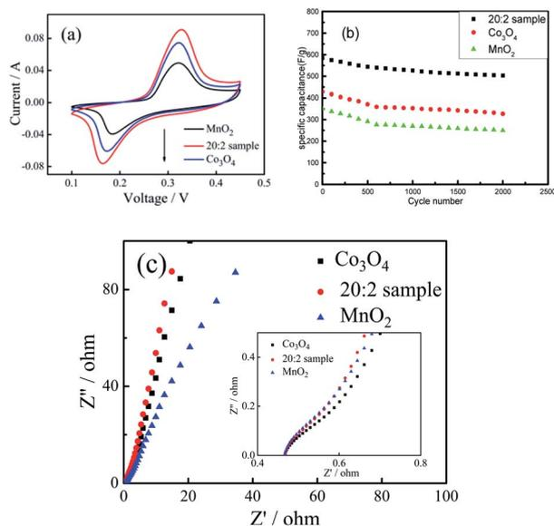
Fig. 7 (a) CV curves for the 20 : 2 sample, pure  $\text{Co}_3\text{O}_4$  nano-fibers and pure  $\text{MnO}_2$  nano-fibers at the scanning rate of  $50 \text{ mV s}^{-1}$ . (b) Cycling stability of the 20 : 2 sample, pure  $\text{Co}_3\text{O}_4$  nano-fibers and pure  $\text{MnO}_2$  nano-fibers at a GCD current density of  $1 \text{ A g}^{-1}$ . (c) AC impedance spectra of the 20 : 2 sample, pure  $\text{Co}_3\text{O}_4$  and pure  $\text{MnO}_2$  nano-fibers.
