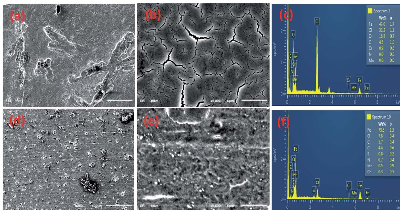
**Fig. 12** (a) low, (b) high SEM image & (c) EDX spectrum of carbon steel surface after 24 hours immersion in the blank solution (d) low, (e) high SEM image & (f) EDX spectrum of carbon steel surface after 24 hours immersion in 600 ppm BSB inhibited solution.
