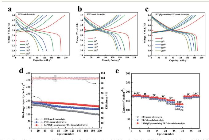
Fig. 3 Charge/discharge curves of  $LiNi_{0.5}Mn_{0.3}Co_{0.2}O_2$  cathodes with the (a) EC-based electrolyte, (b) FEC-based electrolyte, and (c)  $LiPO_2F_2$ -containing the FEC-based electrolyte at voltages ranging from 3.0 to 4.4 V. (d) Cycling performances and coulombic efficiencies of  $LiNi_{0.5}Mn_{0.3}Co_{0.2}O_2$  cathodes with various electrolytes between 3.0 and 4.4 V. (e) Rate capability of  $LiNi_{0.5}Mn_{0.3}Co_{0.2}O_2$  cathodes in various electrolytes.
