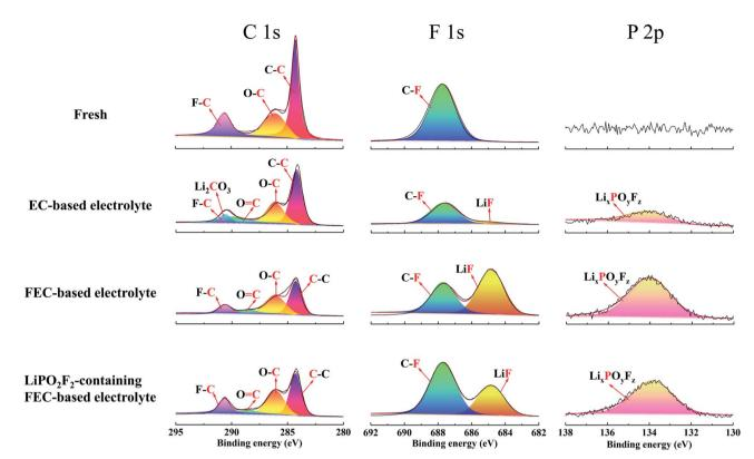
Fig. 6 The C 1s, F 1s, and P 2p spectra of the LiNi $_{0.5}$ Mn $_{0.3}$ Co $_{0.2}$ O $_{2}$  cathodes using various electrolytes obtained after 50 cycles. The XPS spectra of the pristine LiNi<sub>0.5</sub>Mn<sub>0.3</sub>Co<sub>0.2</sub>O<sub>2</sub> cathode are compared.
