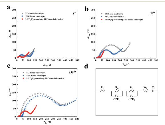
Fig. 4 Nyquist plots of LiNi $_{0.5}$ Mn $_{0.3}$ Co $_{0.2}$ O $_2$ /Li cells in various electrolytes: (a) after 1 cycle, (b) after 50 cycles, and (c) after 150 cycles, respectively. (d) The corresponding equivalent circuit model.
