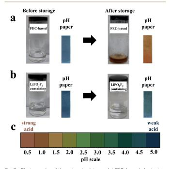
Fig. 7 Photographs of the solvent mixtures: (a) FEC-based electrolyte with 300 ppm  $H_2O$  before and after storage for 3 days. (b) LiPO<sub>2</sub>F<sub>2</sub>containing FEC-based electrolyte with 300 ppm H<sub>2</sub>O before and after storage for 3 days. (c) Indicator chart for the pH scale.
