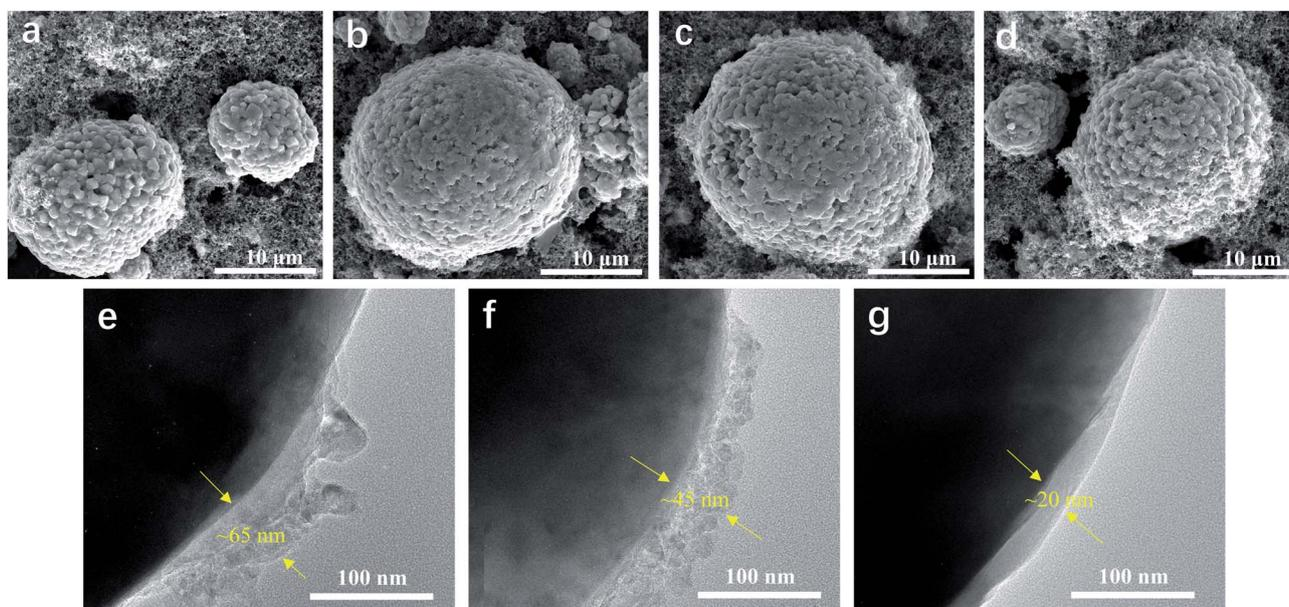
Fig. 5 SEM images of (a) pristine and cycled  $\text{LiNi}_{0.5}\text{Mn}_{0.3}\text{Co}_{0.2}\text{O}_2$  electrodes with (b) the EC-based electrolyte, (c) FEC-based electrolyte, and (d)  $\text{LiPO}_2\text{F}_2$ -containing the FEC-based electrolyte after 100 cycles. TEM images of cycled cathodes with (e) the EC-based electrolyte, (f) FEC-based electrolyte, and (g)  $\text{LiPO}_2\text{F}_2$ -containing FEC-based electrolyte after 100 cycles.
