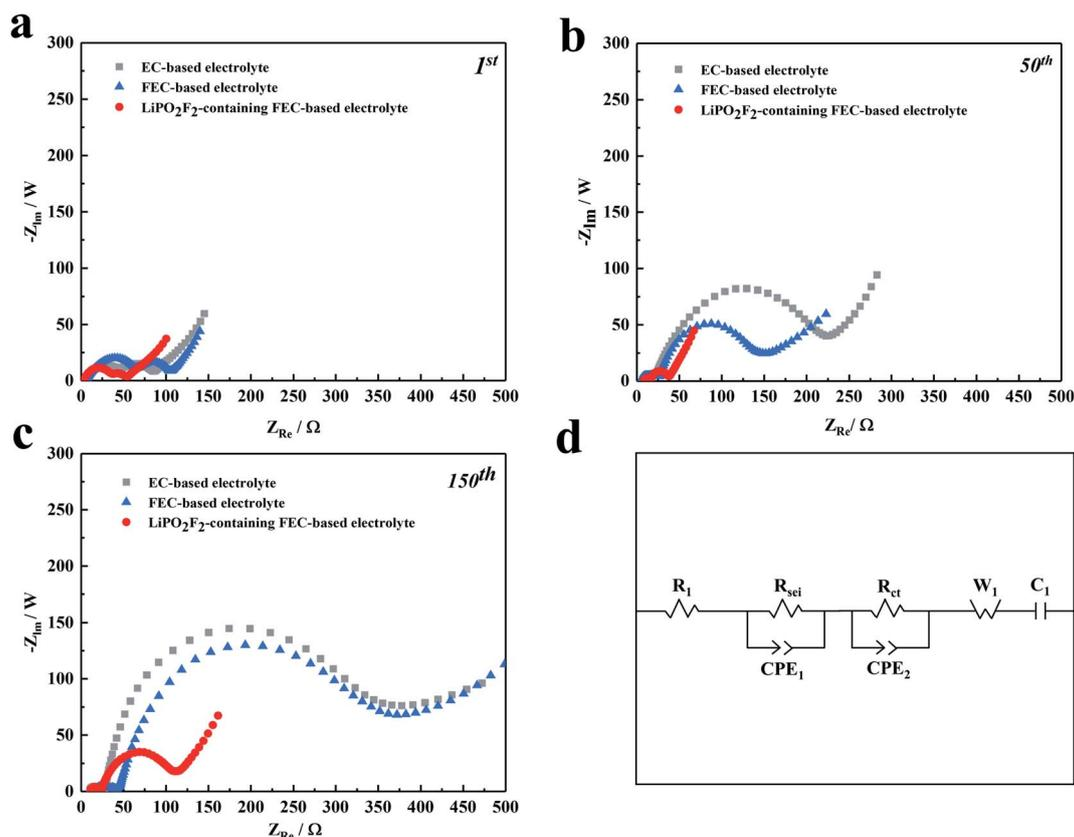
Fig. 4 Nyquist plots of  $\text{LiNi}_{0.5}\text{Mn}_{0.3}\text{Co}_{0.2}\text{O}_2/\text{Li}$  cells in various electrolytes: (a) after 1 cycle, (b) after 50 cycles, and (c) after 150 cycles, respectively. (d) The corresponding equivalent circuit model.
