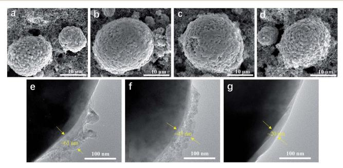
Fig. 5 SEM images of (a) pristine and cycled  $LiNi_{0.5}Mn_{0.3}Co_{0.2}O_2$  electrodes with (b) the EC-based electrolyte, (c) FEC-based electrolyte, and (d) LiPO<sub>2</sub>F<sub>2</sub>-containing the FEC-based electrolyte after 100 cycles. TEM images of cycled cathodes with (e) the EC-based electrolyte, (f) FEC-based electrolyte, and (g) LiPO<sub>2</sub>F<sub>2</sub>-containing FEC-based electrolyte after 100 cycles.
