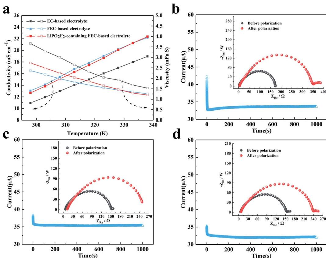
Fig. 2 (a) Conductivity and viscosity of the electrolyte solution: EC-based electrolyte, FEC-based electrolyte and  $\text{LiPO}_2\text{F}_2$ -containing FEC-based electrolyte. Chronopotentiometry for (b) EC-based electrolyte, (c) FEC-based electrolyte, and (d)  $\text{LiPO}_2\text{F}_2$ -containing FEC-based electrolyte.
