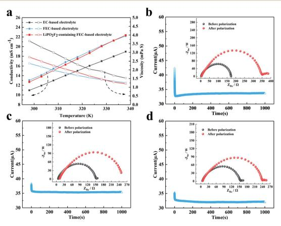
Fig. 2 (a) Conductivity and viscosity of the electrolyte solution: EC-based electrolyte, FEC-based electrolyte and LiPO $_2$ F $_2$ -containing FEC-based electrolyte. Chronopotentiometry for (b) EC-based electrolyte, (c) FEC-based electrolyte, and (d) LiPO $_2$ F $_2$ -containing FEC-based electrolyte.
