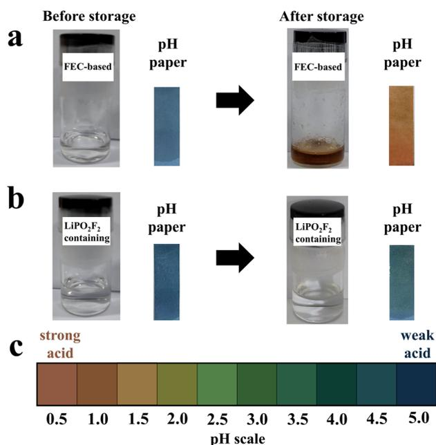
Fig. 7 Photographs of the solvent mixtures: (a) FEC-based electrolyte with 300 ppm H<sub>2</sub>O before and after storage for 3 days. (b) LiPO<sub>2</sub>F<sub>2</sub>-containing FEC-based electrolyte with 300 ppm H<sub>2</sub>O before and after storage for 3 days. (c) Indicator chart for the pH scale.
