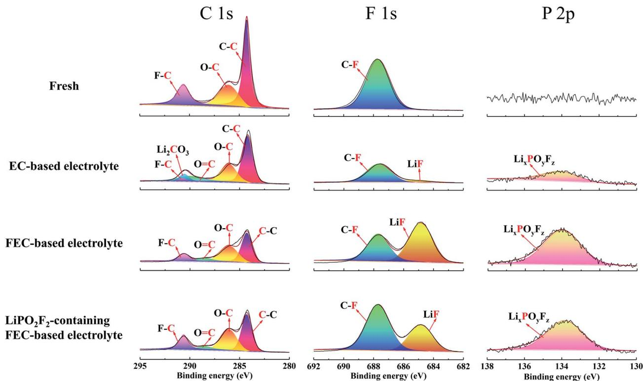
Fig. 6 The C 1s, F 1s, and P 2p spectra of the LiNi<sub>0.5</sub>Mn<sub>0.3</sub>Co<sub>0.2</sub>O<sub>2</sub> cathodes using various electrolytes obtained after 50 cycles. The XPS spectra of the pristine LiNi<sub>0.5</sub>Mn<sub>0.3</sub>Co<sub>0.2</sub>O<sub>2</sub> cathode are compared.
