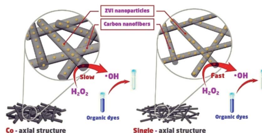
Scheme 1 The speculated degradation mechanism of MB catalysed by as-prepared carbon nanofibrous mats with either the single-axial or co-axial structure.
