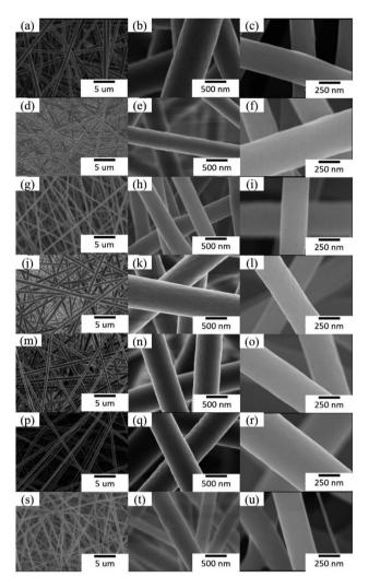
Fig. 1 SEM images of as-prepared nanofibrous mats before (left two lanes) and after annealing treatment (right lane). (a and b) S1, (c) S1-a, (d and e) S2, (f) S2-a, (g and h) S3, (i) S3-a, (j and k) C1, (l) C1-a, (m and n) C2, (o) C2-a, (p and q) C3, (r) C3-a, (s and t) S0, (u) S0-a.
