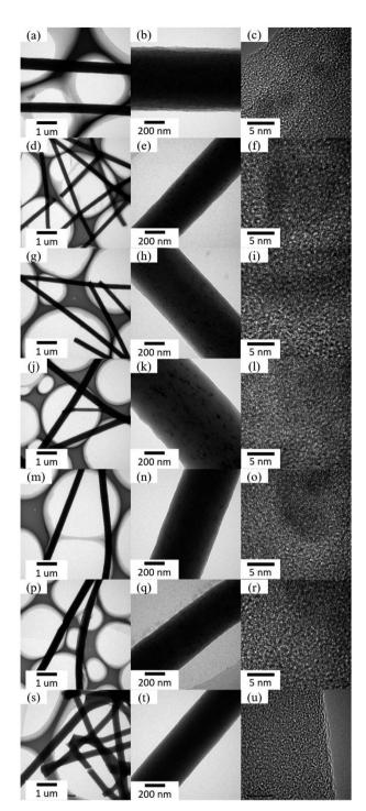
Fig. 3 TEM and HRTEM images of as-prepared nanofibrous mats after annealing treatment. (a–c) S1-a, (d–f) S2-a, (g–i) S3-a, (j–l) C1-a, (m–o) C2-a, (p–r) C3-a, and (s–u) S0-a.
