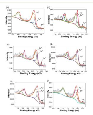
Fig. 4 XPS spectra of Fe 2p in as-prepared nanofibrous mats after annealing treatment. (a) S1-a, (b) S2-a, (c) S3-a, (d) C1-a, (e) C2-a, (f) C3-a.
