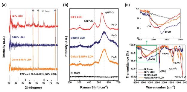
Fig. 3 Structural characterization and spectral analysis to confirm successful gaseous boronization and electrochemical oxidation. (a) X-ray diffraction (XRD) analysis for verification of electrochemical oxidation and boronization. (b) Raman spectral analysis of the NiFe LDH-based electrocatalysts. (c) Fourier transformation infrared (FT-IR) spectral analysis to confirm boron doping of NiFe LDH.
