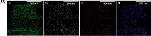
Fig. 2 Further morphological characterization of B:NiFe LDH before and after galvanostatic oxidation. (a) Transmission Electron Microscopy (TEM) analysis (top of each row) and selected area electron diffraction (SAED) pattern (bottom of each row) of the NiFe LDH-based electrocatalyst under each condition. (b) EDS mapping of TEM images of the B:NiFe LDH chemical composition
