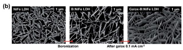
Fig. 1 Summary of the fabrication scheme and structural and morphological characterization of galvanostatic oxidized nickel-iron layered double hydroxide (NiFe LDH) with boron doping. (a) Schematic illustration of the synthesis of galvanostatic oxidized boron-doped NiFe LDH (galox-B:NiFe LDH) through gas-solid boronization in a furnace and electrochemical oxidation. (b) Field-emission scanning electron microscopy (FE-SEM) images of the NiFe LDH-based electrocatalyst under each condition.
