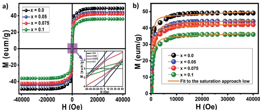
Fig. 8 Magnetic hysteresis loops obtained for the nanocrystalline undoped and neodymium-doped Ni-Zn-Al ferrite ( $Ni_{0.6}Zn_{0.4}Al_{0.5}Fe_{1.5-x}Nd_xO_4$ ) powders (a) and  $M-H$  variation curves (b).
