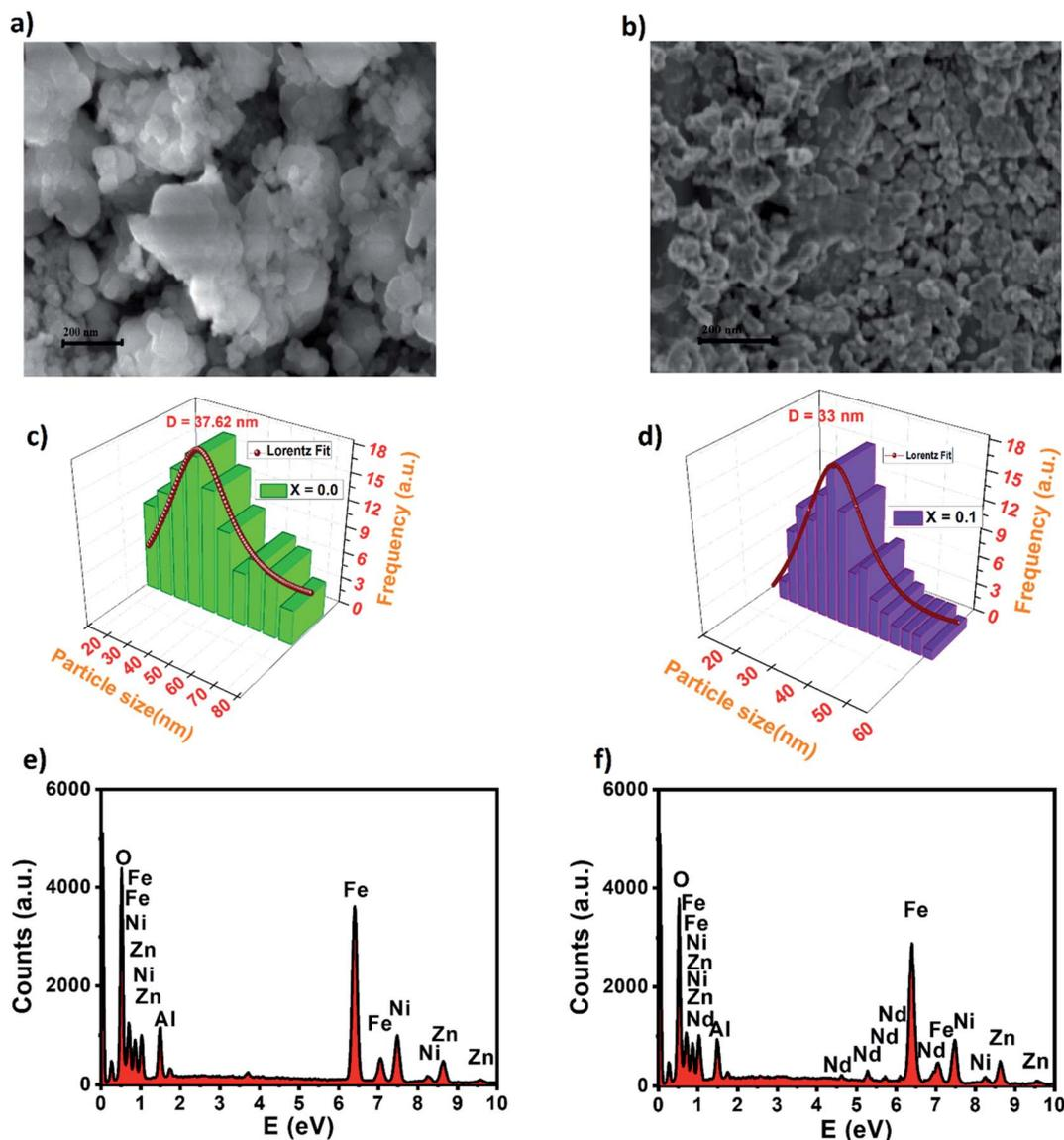
Fig. 3 SEM micrograph of nickel-zinc ferrites for (a)  $x = 0.00$ , (b)  $x = 0.1$ , particle size distribution for (c)  $x = 0.00$  and (d)  $x = 0.1$  and EDX spectrum of (e)  $x = 0.00$  and (f)  $x = 0.1$ .
