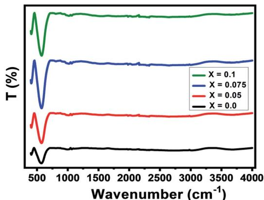
Fig. 4 FTIR transmittance spectra of  $\text{Nd}^{3+}$  doped Ni-Zn ferrites.
