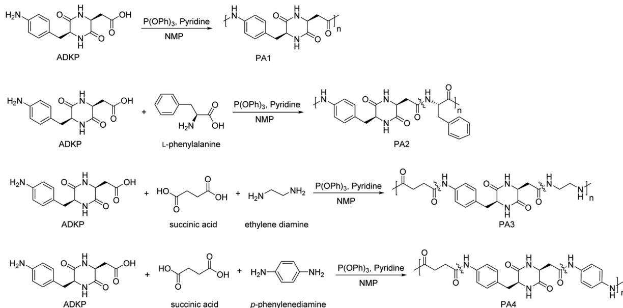
Scheme 2 Synthesis of DKP-based polyamides from cyclo(L-aspartyl-4-amino-L-phenylalanyl).
