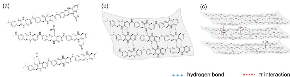
Fig. 4 Schematic illustration of formation of (a) irregular gel-like morphologies, (b) sheet-like substructure and (c) cubic particles.
