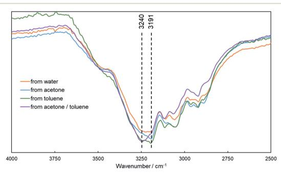
Fig. 3 IR spectra of PA1 particles precipitated from water, acetone, toluene, and mixture of acetone/toluene.
