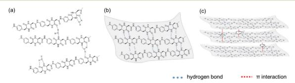
Fig. 4 Schematic illustration of formation of (a) irregular gel-like morphologies, (b) sheet-like substructure and (c) cubic particles.
