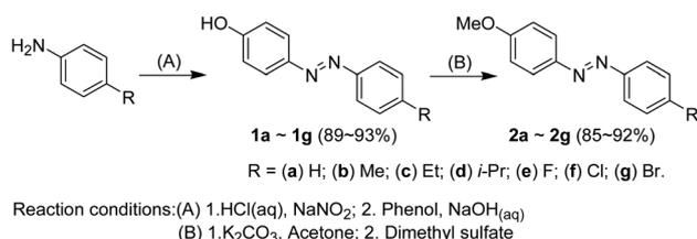
Scheme 2 The synthesis of the 4-methoxy-4'-substituted azobenzenes **2a–2g**.
