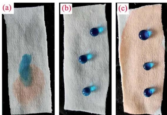
Fig. 9 (a) Photograph of water (dyed with MB) and dichloromethane (dyed with OR) on a pristine textile. (b) Photograph of water droplets on  $\text{SiO}_2\text{-S-PIH@cotton}$ . (c) Photograph of water droplets and *n*-hexane on  $\text{SiO}_2\text{-S-PIH@cotton}$ .
