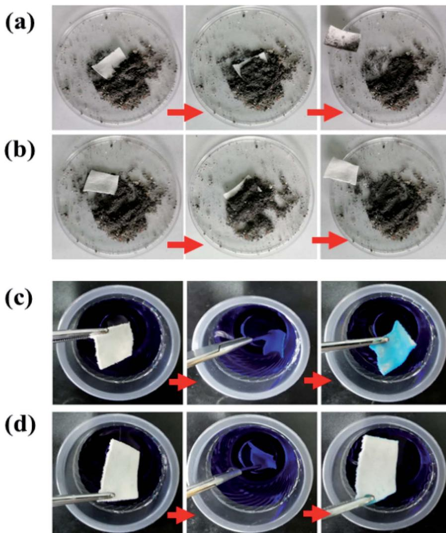
Fig. 8 Self-cleaning ability of (a) pristine cotton textile and (b) SiO<sub>2</sub>-S-PIH@ cotton with powder contaminants. Self-cleaning ability of (c) pristine cotton textile and (d) SiO<sub>2</sub>-S-PIH@ cotton in polluted solutions.
