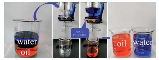
Fig. 11 Photographs of the oil-water separation process with SiO<sub>2</sub>-S-PIH@cotton.
