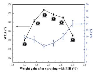
Fig. 5 The WCAs and SAs of cottons with different weight gains after spraying with PIH.
