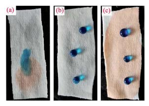
Fig. 9 (a) Photograph of water (dyed with MB) and dichloromethane (dyed with OR) on a pristine textile. (b) Photograph of water droplets on  $SiO_2$ -S-PIH@cotton. (c) Photograph of water droplets and nhexane on SiO<sub>2</sub>-S-PIH@cotton.
