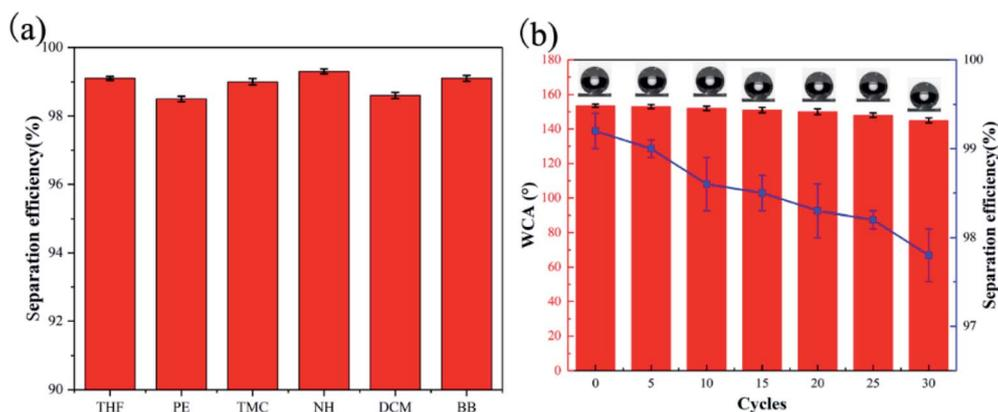
Fig. 12 (a) The separation efficiency of  $\text{SiO}_2\text{-S-PIH@ cotton}$  for various oil–water mixtures. (b) The variation of separation efficiency and WCA of  $\text{SiO}_2\text{-S-PIH@ cotton}$  versus the number of separation cycles.
