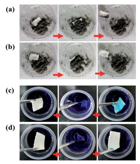
Fig. 8 Self-cleaning ability of (a) pristine cotton textile and (b)  $SiO_2 - S - PIH$ @cotton with powder contaminants. Self-cleaning ability of (c) pristine cotton textile and (d)  $SiO_2 - S - PIH$ @cotton in polluted solutions.
