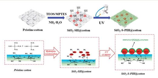
Scheme 1 Preparation of SiO<sub>2</sub>-SH@cotton and SiO<sub>2</sub>-S-PIH@cotton.
