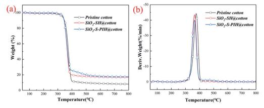
Fig. 2 The TGA (a) and DTG (b) curves of pristine cotton, SiO<sub>2</sub>-SH@cotton and SiO<sub>2</sub>-S-PIH@cotton under a N<sub>2</sub> atmosphere
