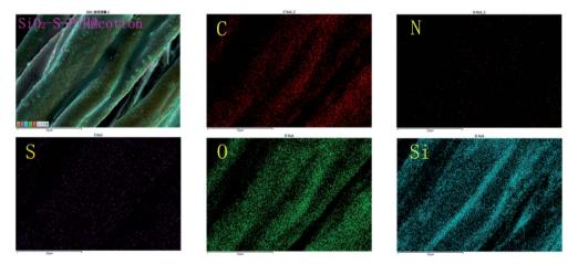
Fig. 4 EDX elemental mapping images of carbon, nitrogen, sulfur, silicon, and oxygen of SiO<sub>2</sub>-S-PIH@cotton at 2000 SE
