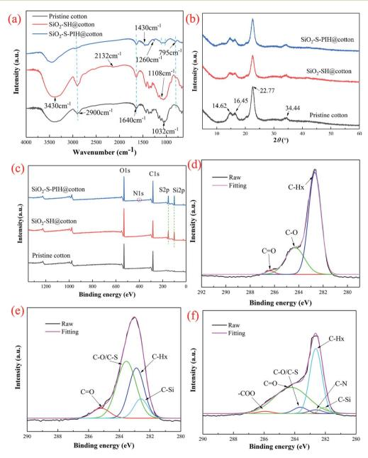
Fig. 1 (a) The FT-IR spectra of pristine cotton fabric,  $SiO_2$ -SH@cotton and  $SiO_2$ -S-PIH@cotton. (b) The XRD of pristine cotton,  $SiO_2$ -SH@cotton and  $SiO_2$ -S-PIH@cotton and  $SiO_2$ -S-PIH@cotton. (c) The XPS spectra of the pristine cotton fabric,  $SiO_2$ -SH@cotton and  $SiO_2$ -S-PIH@cotton. The high-resolution XPS spectra of the C 1s region of (d) pristine cotton fabric, (e)  $SiO_2$ -SH@cotton and (f)  $SiO_2$ -S-PIH@cotton.
