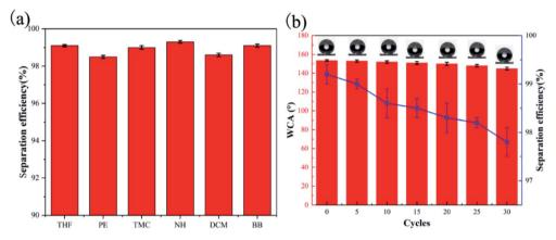
Fig. 12 (a) The separation efficiency of  $SiO_2$ –S–PIH@cotton for various oil–water mixtures. (b) The variation of separation efficiency and WCA of  $SiO_2$ –S–PIH@cotton *versus* the number of separation cycles.
