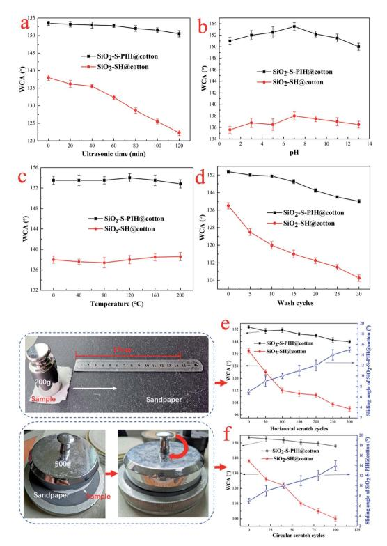
Fig. 7 The influence of (a) ultrasonic treatment, (b) solutions with different pH values, (c) placed under different temperatures for 6 h, and (d) wash cycles. Effect of (e) horizontal scratch cycles, and (f) circular scratches, on WCAs and SAs of SiO<sub>2</sub>-SH@cotton and SiO<sub>2</sub>-S-PIH@cotton.
