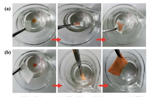
Fig. 10 Absorption processes of (a) light oil (n-hexane, dyed with OR) and (b) heavy oil (dichloromethane, dyed with OR) from water using SiO<sub>2</sub>-S-PIHacotton.
