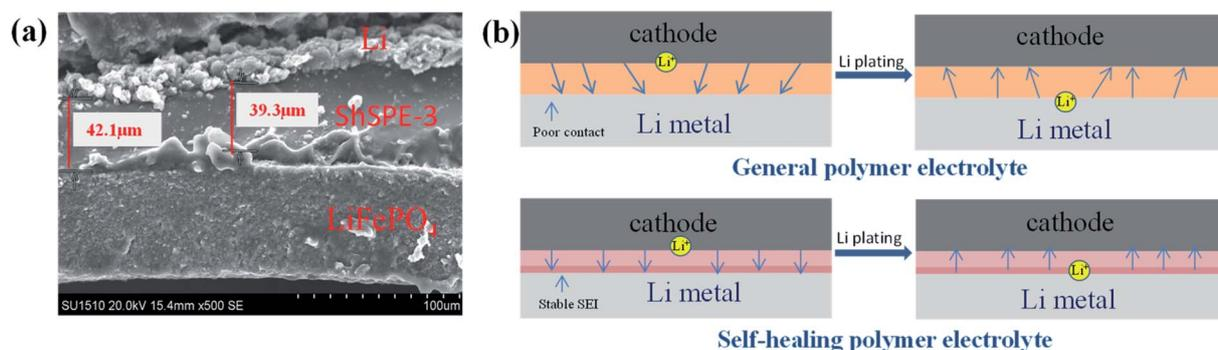
Fig. 7 Cross-sectional SEM images of the Li/ShSPE-3/LiFePO<sub>4</sub> (a) and schematic illustration of Li plating of general and self-healing polymer electrolytes on Li metal (b).
