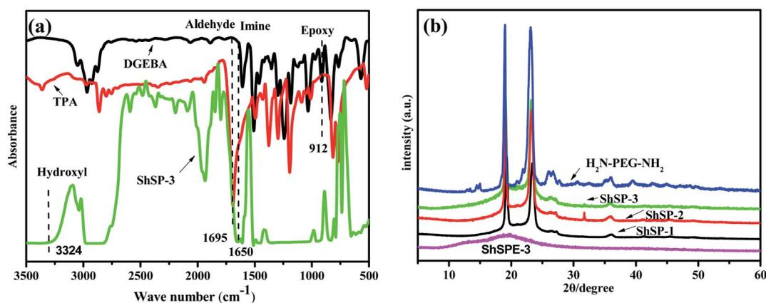
Fig. 3 FT-IR spectra of DGEBA, TPA and ShSP-3 elastomer (a) and XRD spectra (b) for  $\text{NH}_2\text{-PEG-NH}_2$ , polymers without Li salts (ShSP-1, 2, 3) and ShSPE-3.
