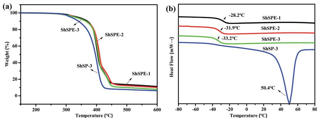
Fig. 4 TGA (a) and DSC (b) curves for self-healable solid polymers without Li salts (ShSP-3) and the self-healable polymeric electrolyte at different molar ratios.
