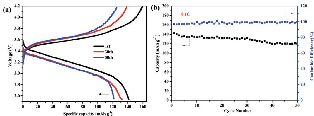
Fig. 9 Charge-discharge curves of ShSPE-3 based LiFePO<sub>4</sub>/Li cell for 0.1C at 60 °C with the voltage range from 2.5 to 4.2 V (a), cycling performance of the LFP/ShSPE-3/Li cell (b).
