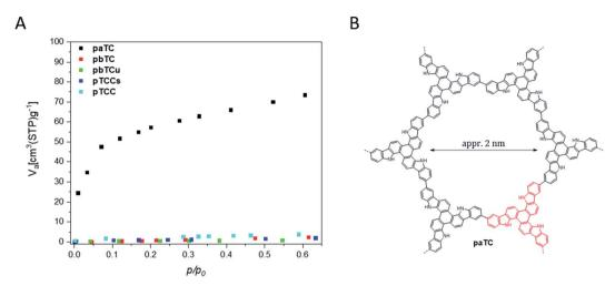
Fig. 4 (A) Krypton gas adsorption isotherms of the electropolymerized films prepared from the tricarbazole monomers. aTC (black), pbTC (red), pbTCu (green), psTCC (blue), pTCC (cyan). (B) Idealized, hexameric macrocyclic pore of paTC.
