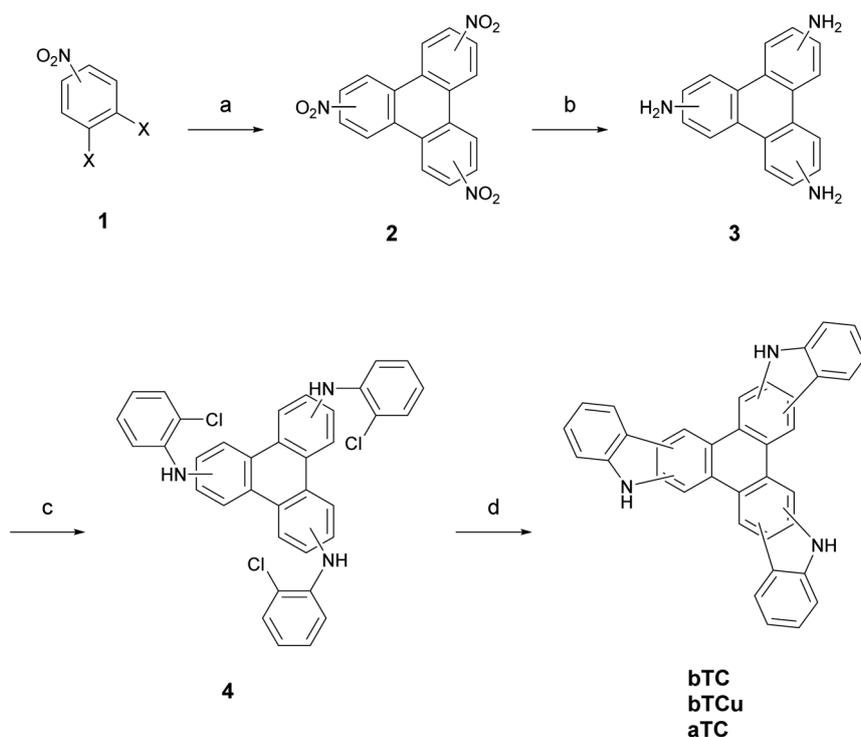
**Scheme 1** General synthetic pathway towards the planar tricarbazole derivatives. (a) Cu, DMF, 200 °C, 12 h; (b) H<sub>2</sub>, Pd/C, ethyl acetate/ethanol (10/1); (c) *t*-BuONa, 1-bromo-2-chlorobenzene, DavePhos-catalyst, 1,4-dioxane, 125 °C, 18 h; (d) DBU, Pd(OAc)<sub>2</sub>, P(*t*-Bu)<sub>3</sub>, *o*-xylene, 140 °C, 18 h. (X = Br or Cl).
