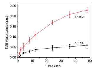
Fig. 7 Detection of 'OH generation in an  $H^+$  enhanced tumor environment (around pH = 5.2).
