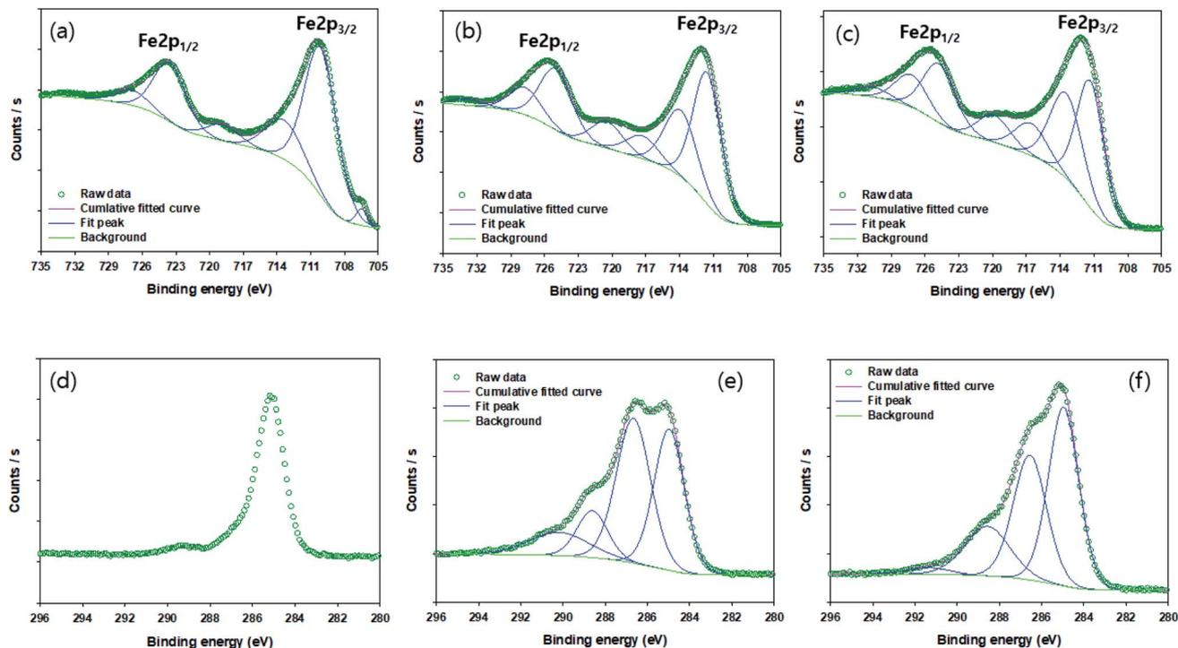
Fig. 2 The XPS spectra of iron and carbon on the surface of NZVI before  $\text{BrO}_3^-$  reduction (a and d), those of G-NZVI before the reaction (b and e), and those of G-NZVI after the reaction (c and f).
