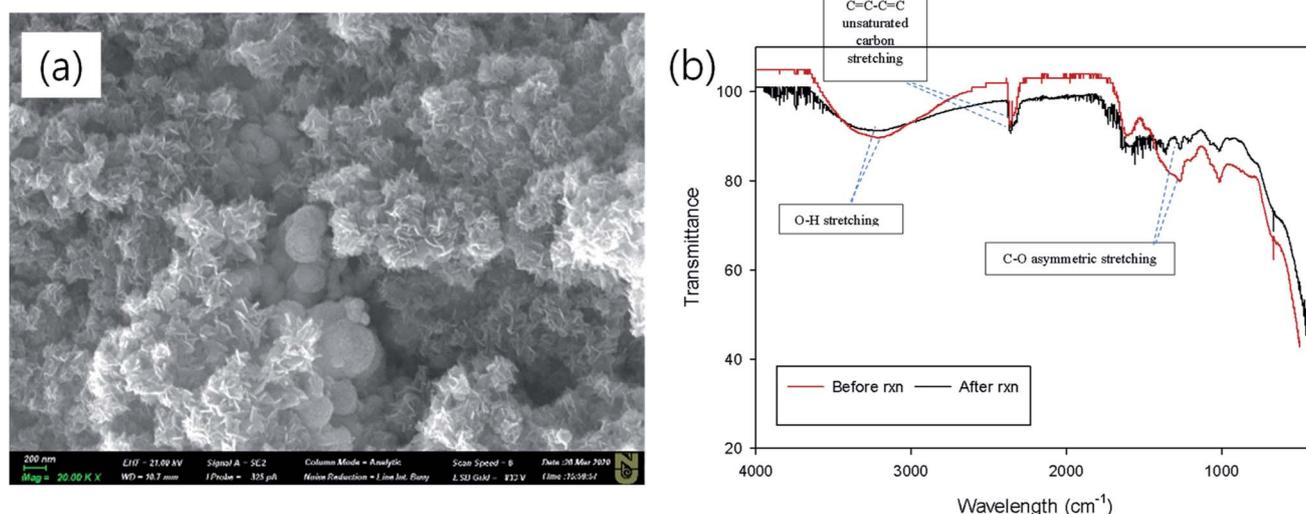
Fig. 7 SEM image (a) and FTIR spectra (b) of G-NZVI after BrO<sub>3</sub><sup>-</sup> reduction.
