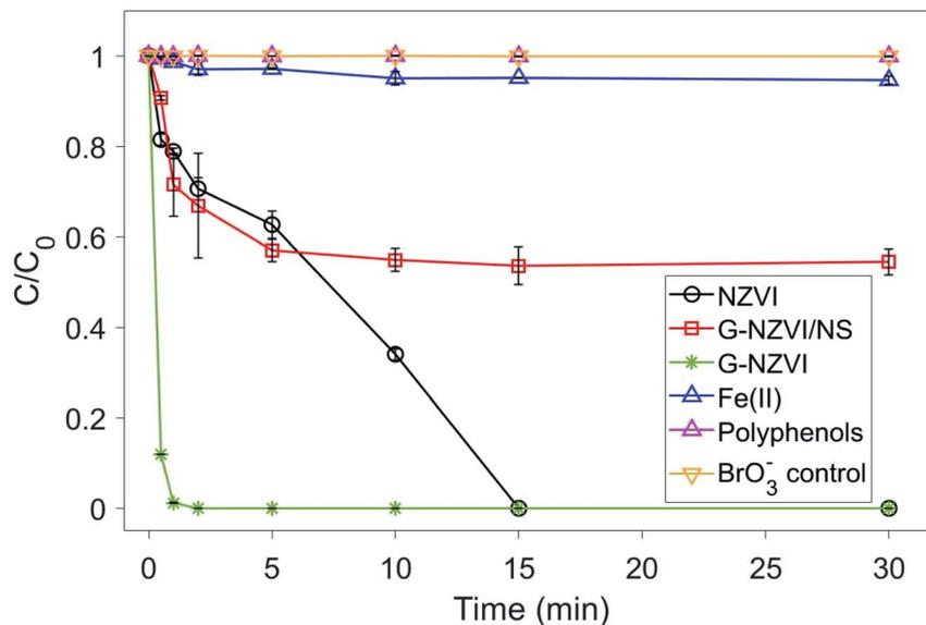
Fig. 5 The  $\text{BrO}_3^-$  reduction kinetics using five types of controls under aerobic conditions. Material loading:  $200 \text{ mg L}^{-1}$  and  $\text{BrO}_3^-$  concentration:  $50 \text{ mg L}^{-1}$ .
