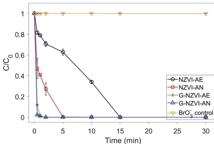
Fig. 6 The  $\text{BrO}_3^-$  reduction kinetics of using G-NZVI and NZVI under aerobic and anaerobic conditions. Material loading:  $200 \text{ mg L}^{-1}$ ,  $\text{BrO}_3^-$  concentration:  $50 \text{ mg L}^{-1}$ .
