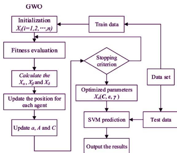
Fig. 3 Flowchart of optimized SVM with GWO algorithm.
