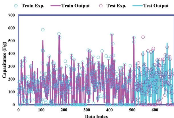
Fig. 5 Experimental *versus* predicted capacitances of the carbon-based EDLCs from the GWO-SVM.
