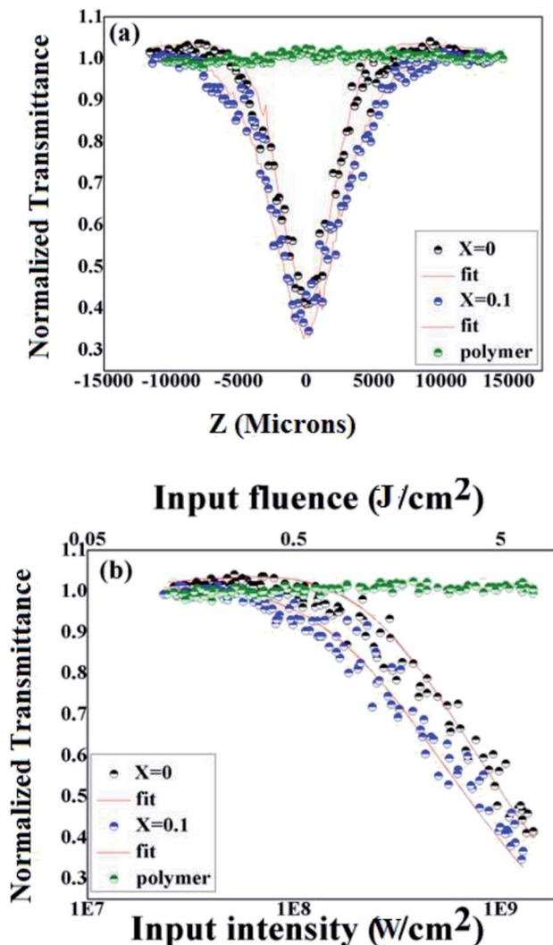
Fig. 4 (a) Open aperture Z-scan curves obtained in PMMA,  $x = 0$  and  $x = 0.1$  compositions for 5 ns pulse excitation. (b) Intensity-dependent normalized transmission in PMMA,  $x = 0$  and  $x = 0.1$  compositions for 5 ns pulse excitation.
