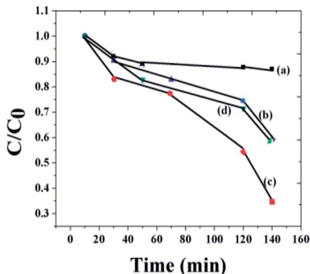
Fig. 7 The degradation process of methyl orange by different photocatalysts: (a)  $x = 0$  composition with 135 nm size, (b)  $x = 0$  composition of 6 nm size, (c)  $x = 0.1$  composition, (d)  $x = 0.5$  composition.
