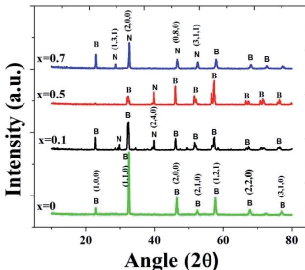
Fig. 1 XRD patterns of (1 – x)BiFeO<sub>3</sub>–xNaNbO<sub>3</sub> composites.
