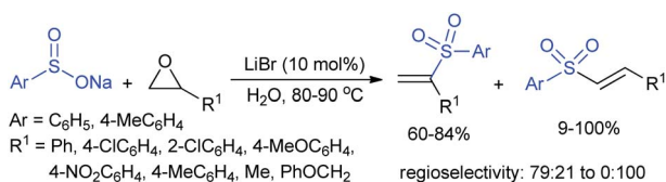
Scheme 78 Synthesis of vinyl sulfones via the opening of epoxides with sodium sulfonates.
