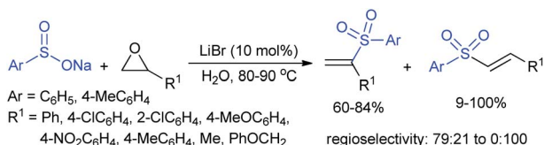
Scheme 78 Synthesis of vinyl sulfones via the opening of epoxides with sodium sulfinates.
