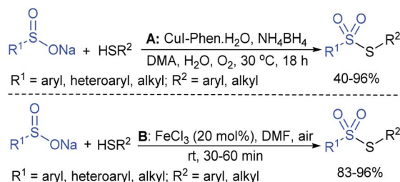
Scheme 17 Sulfenylation of thiols with sodium sulfinates.
