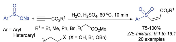
Scheme 102 Sulfonylation of propargylic carboxylates with sulfinates.
