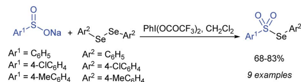
Scheme 21 Synthesis of selenosulfonates from diaryl diselenides with sodium sulfonates.
