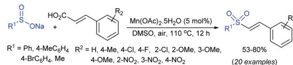
Scheme 118 Decarboxylative coupling of cinnamic acids with sulfonate salts.
