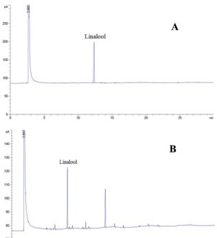
Fig. 2 GC chromatograms of linalool (A) and lavender oil (B) (linalool  $\mathsf{RT}=12.34$  min).
