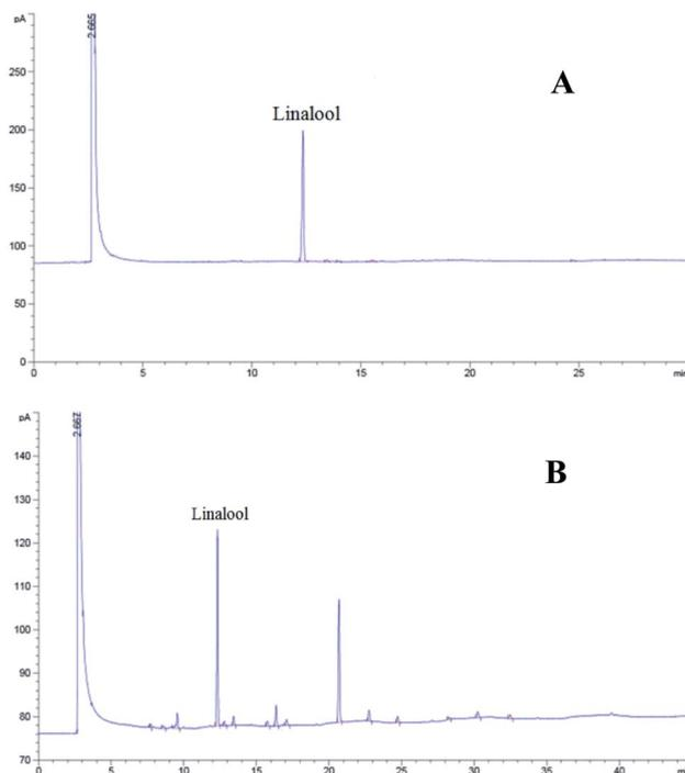
Fig. 2 GC chromatograms of linalool (A) and lavender oil (B) (linalool RT = 12.34 min).
