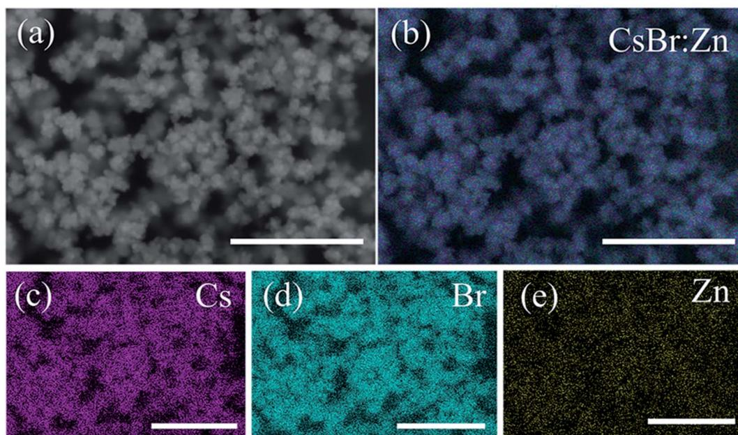
Fig. 2 Elemental characterization of CsBr:Zn NCs. (a) SEM image of CsBr:Zn NCs. (b) EDS mapping of CsBr:Zn NCs. (c–e) Corresponding elemental mapping of Cs, Br, and Zn in CsBr:Zn NCs. Scale bars are 5  $\mu\text{m}$  in all images.
