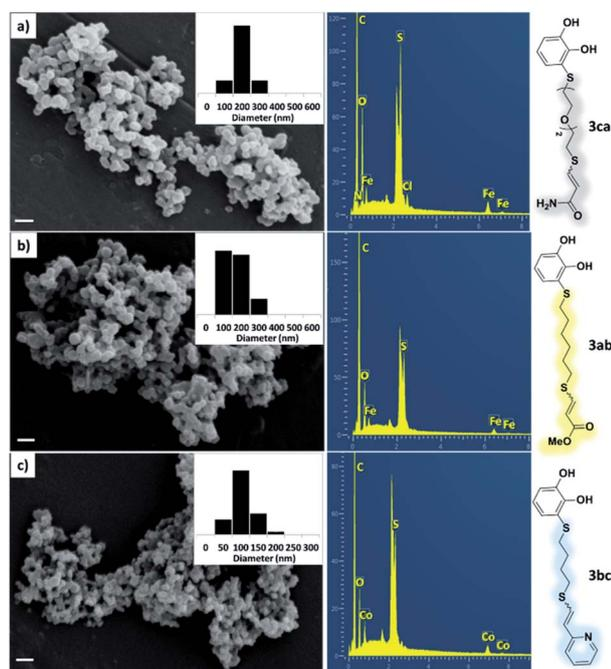
Fig. 2 SEM micrographs, histograms and EDX spectra for CNPs prepared by mixing: (a) **3ca** ligand with  $\text{Fe(III)}$ , (b) **3ab** ligand with  $\text{Fe(III)}$  and (c) **3bc** ligand with  $\text{Co(II)}$ . Scale bars are 500 nm.
