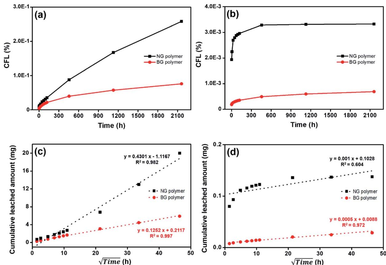
Fig. 3 Leaching behavior of (a and c) Cs and (b and d) Co from NG and BG polymer waste forms. The data were collected up to 90 d (2160 h).
