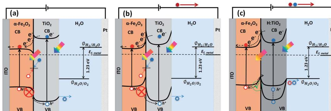
Fig. 1 Approximate energy band diagram and charge transfer mechanism of (a) Fe<sub>2</sub>O<sub>3</sub>-TiO<sub>2</sub> photoanode without external applied anodic potential, (b) Fe<sub>2</sub>O<sub>3</sub>-TiO<sub>2</sub> photoanode with external applied anodic potential and (c) Fe<sub>2</sub>O<sub>3</sub>-H:TiO<sub>2</sub> photoanode with external applied anodic potential.
