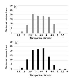
Fig. 6 Size distribution of nanoparticles captured on the graphene membrane (a) on the quartz holder and (b) on the stainless-steel holder.
