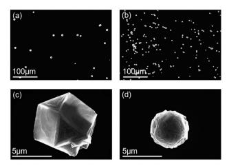
Fig. 7 FESEM images of diamonds deposited for 8 h on the bare silicon substrate (a) on the sapphire plate on the stainless-steel holder and (b) on the stainless-steel holder. (c) and (d) are magnified images of a diamond particle of (a) and (b), respectively.
