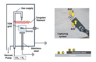
Fig. 1 Schematics of the experimental apparatus for capturing carbon nanoparticles. The left figure is the HWCVD reactor with a capturing apparatus. The right figure illustrates how the SiO and carbon membranes are made electrically floating and grounded. Nanoparticles were captured on floating and grounded SiO and carbon membranes under the same HFCVD condition. 'S' and 'C' in the right figure indicate SiO and carbon membranes, respectively.
