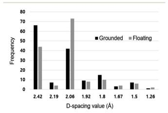
Fig. 5 Frequency of d-spacing values of nanoparticles captured at 1% CH<sub>4</sub>-99% H<sub>2</sub>. The data were obtained by analyzing 150 d-spacing values out of  $\sim$ 100 nanodiamonds for each membrane.
