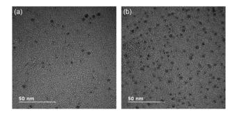
Fig. 3 TEM images of nanoparticles captured on the graphene membrane of the TEM Cu grid (a) on the quartz holder and (b) on the stainless-steel holder at the capture temperature of 600  $^{\circ}$ C and the gas mixture of 1% CH<sub>4</sub>–99% H<sub>2</sub>.
