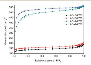
Fig. 3 N<sub>2</sub> adsorption and desorption isotherms of the AC samples.
