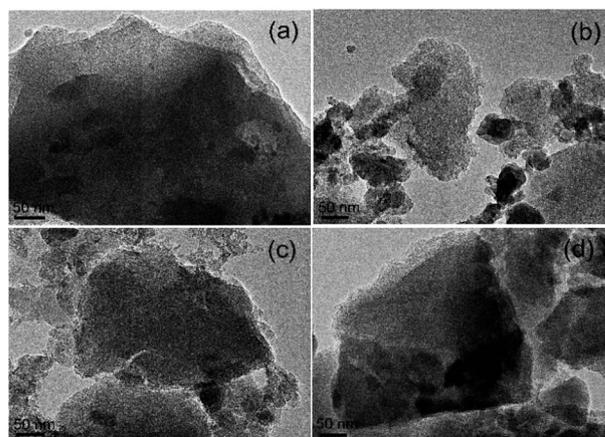
Fig. 2 TEM images of (a) AC-1.0-700, (b) AC-2.0-700, (c) AC-3.0-700 and (d) AC-4.0-700.
