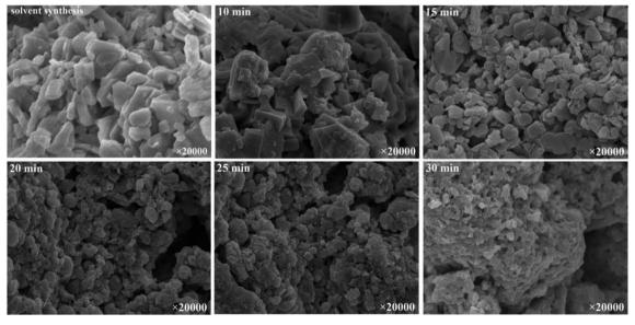
Fig. 2 SEM images of the Zn-Co DMC catalyst samples.
