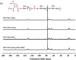
Fig. 8  $^{1}$ H and  $^{13}$ C NMR spectra of the tercopolymer PPCTMA synthesized by using ZnGA/RET/DMC as the catalyst.
