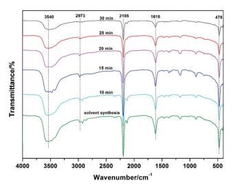
Fig. 3 Comparisons of the FTIR spectra of the Zn–Co DMC samples synthesized for the specified time.
