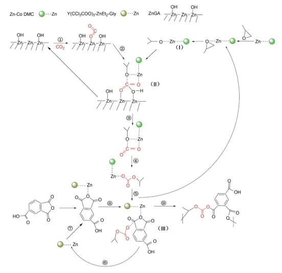
Scheme 2 Proposed mechanism of the CO<sub>2</sub>/PO/TMA terpolymerization over the ZnGA/RET/DMC composite catalyst system.
