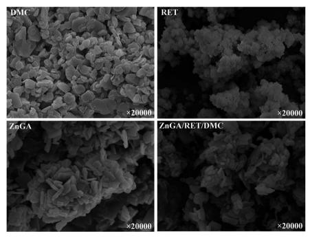
Fig. 5 SEM images of the DMC, RET, ZnGA and ZnGA/RET/DMC composite catalyst samples.
